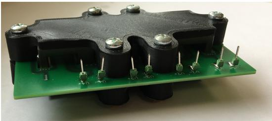
Fig. 10: Experimental Inter Cell Transformer
