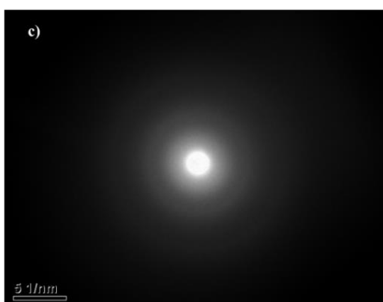
Figure S2. a): SEM image; b): EDS analysis; and c): ED pattern of Cu@C catalyst.
