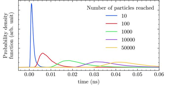
Fig. 10. Distribution of the time between the first impact ionization event and different number of particles thresholds. This figure illustrates the timing jitter due to the avalanche process itself. There is a not negligible spread of time for the avalanche to be established at measurable levels of currents.
