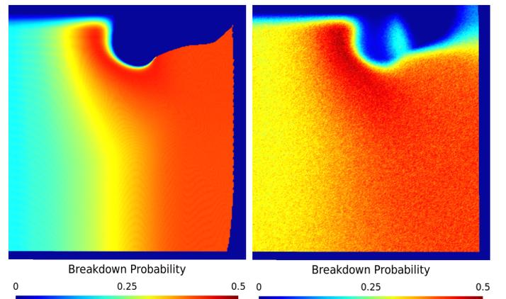
Fig. 8. Two-dimensional map of breakdown probability obtained by the method of Hellebois and al. using the McIntyre model over electric field lines [28] (left). Two-dimensional map of breakdown probability obtained from the ADMC method (right).
