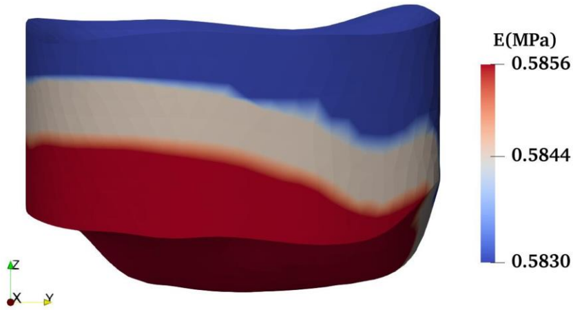
Figure 12 Target Young's modulus distribution of the LC case.
