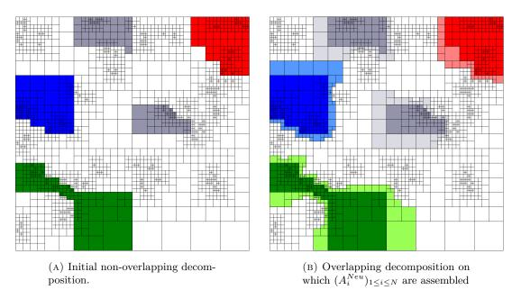
FIGURE 5.3. Automatic generation of overlapping subdomains and assembly of local Neumann operators needed by (4.4). For clarity, only four subdomains, one of which is disconnected, are colored. Figure taken from [23]
