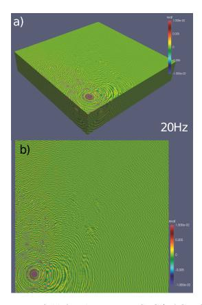
Figure 5.2. 20 Hz wavefield for the acoustic SEG/EAGE Overthrust model computed using P3 finite elements on an unstructured mesh adapted to the local wavelength, with 5 points per wavelength – FreeFem software
