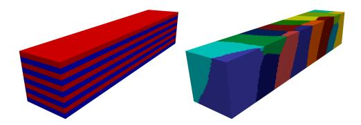
FIGURE 5.1. Heterogeneous beam composed of 10 alternating layers of rubber material  $(E_1, \nu_1) = (1.10^7, 0.4999)$  and steel material  $(E_2, \nu_2) = (210^9, 0.35)$ . Coefficient distribution (left) and mesh partitioning into 16 subdomains by the automatic graph partitioner *Metis* (right).
