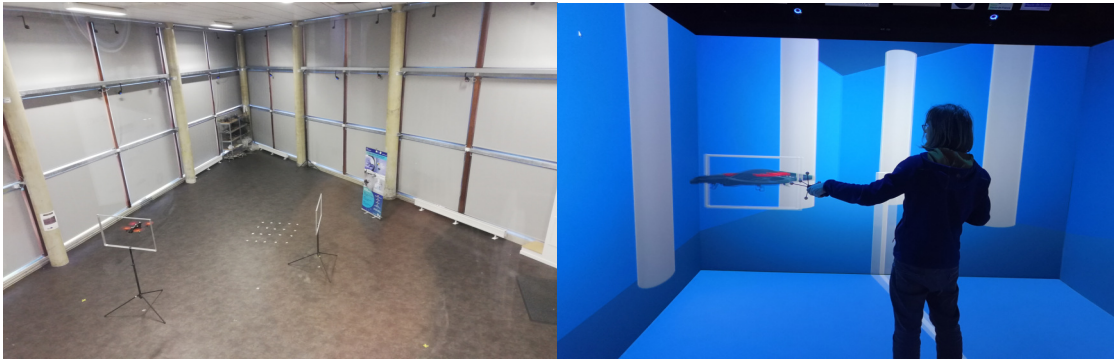
Fig. 6: Left: Real world (flight arena). Right : DrEAM's virtual environment. Observe, in the right picture, that user is in DrEAM piloting the virtual drone for passing through a virtual window, and note in left figure that the real drone is crossing also the 'real' window in autonomous mode without knowing the obstacle position.
