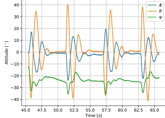
(b) Euler angles equivalent representation of the attitude tracking performance using SSC.
