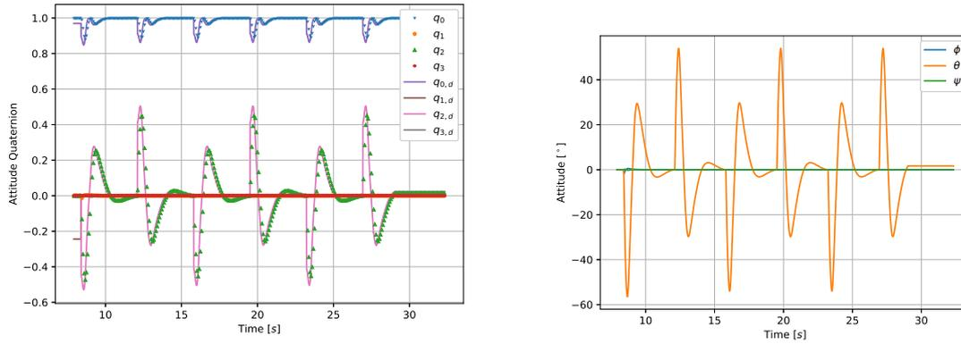
(a) Quaternion reference tracking when using (51). (b) Euler angles equivalent representation of the attitude tracking performance.
