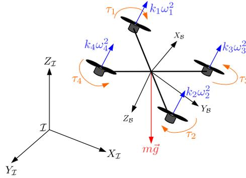
Figure 1.: Quadcopter configuration. Each rotor produces a force  $f_i \sim k_i\omega_i^2$ ; where  $k_i$  is a constant aerodynamic parameter and  $\omega_i$  denotes the angular rate of motor  $i$ .  $\tau_i$  introduces the torque produced by motor  $i$ .  $\mathcal{I} = X_I, Y_I, Z_I$  signifies the inertial frame and  $X_B, Y_B, Z_B$  means the body frame.
