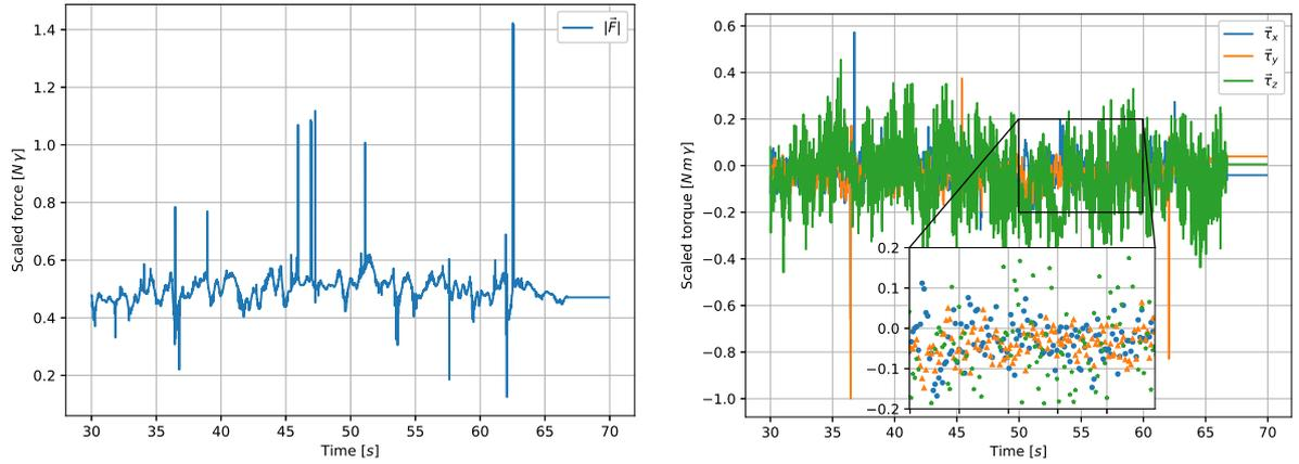
(a) Thrust force performance obtained from the virtual control inputs. (b) Control torques applied to the aerial platform.
