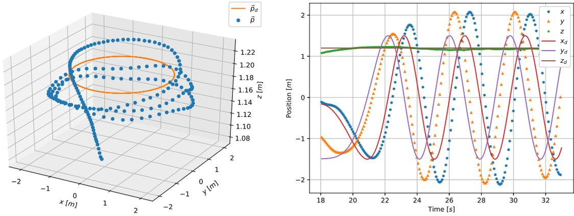
(a) 3D system performance when tracking a circular trajectory. (b) Real-time position behavior of the system.
