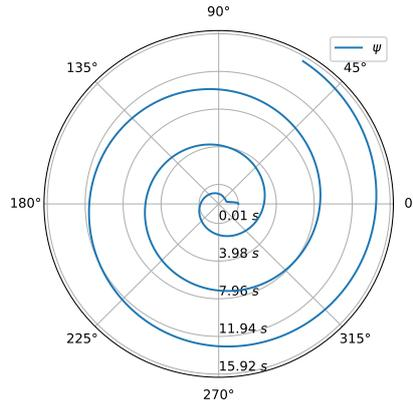
Figure 9.: Quadcopter yaw  $\psi$  attitude for the simulation of scenario A using the separated saturations controller (84). The angle is shown using a polar plot in order to showcase the circle maneuver. The radius of the plot represents time in seconds.
