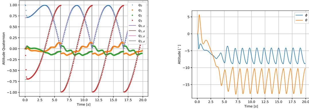
(a) Quaternion reference tracking when using the SSC algorithm. (b) Euler angles roll  $\phi$  and pitch  $\theta$  equivalent representation of the attitude tracking performance using SSC.
