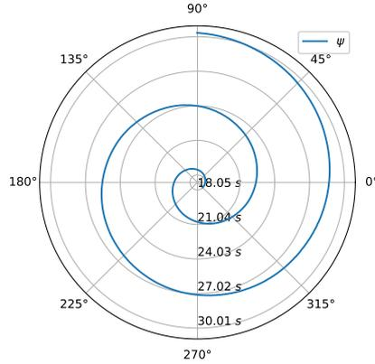
Figure 18.: Quadcopter yaw  $\psi$  attitude for the experiments of scenario A using the separated saturations controller (84). The angle is shown using a polar plot in order to showcase the circle maneuver. The radius of the plot represents time in seconds.
