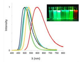
Figure 7. Emission of dye 8 (light blue), 10 (blue), 11 (navy blue), 12 (green), 13 (light green), 15 (orange), and 16 (red) in dichloromethane at 25 °C. (Insert) Photographs of solutions of dyes 8, 10-13 and 15-16 in dichloromethane under irradiation from a bench UV-lamp ( $\lambda_{exc} = 365$  nm).
