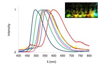
**Figure 3**. Emission in the solid-state, as embedded in KBr pellets (concentration of around  $10^{-4}$  M) of **1** (green), **2** (yellow), **3** (purple), **4** (pink), **5** (blue), **6** (red), **7** (orange), and **8** (navy blue). (Insert) Photographs of solutions of dyes **1-8** as powders under irradiation from a bench UV-lamp ( $\lambda_{exc} = 365$  nm).
