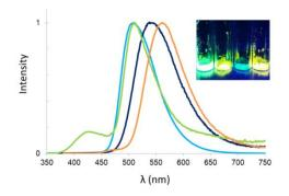
**Figure 8**. Emission in the solid-state, as embedded in KBr pellets (concentration of around  $10^{-4}$  M) of **10** (blue), **11** (navy blue), **13** (light green), and **15** (orange). (Insert) Photographs of solutions of dyes **10**, **11**, **13** and **15** as powders under irradiation from a bench UV-lamp ( $\lambda_{exc} = 365$  nm).
