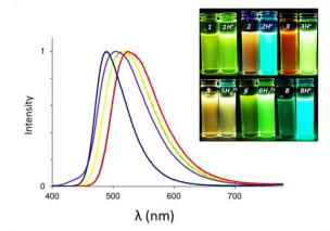
Figure 4. Emission spectra of 1 (green), 2 (yellow), 3 (purple), 5 (blue), 6 (red), 8 (navy blue) in their protonated state in dichloromethane at 25°C. (Insert) Photopgraphs of solution in neutral (left) and protonated (right) dichloromethane under irradiation from a bench UV-lamp ( $\lambda_{exc} = 365$  nm).
