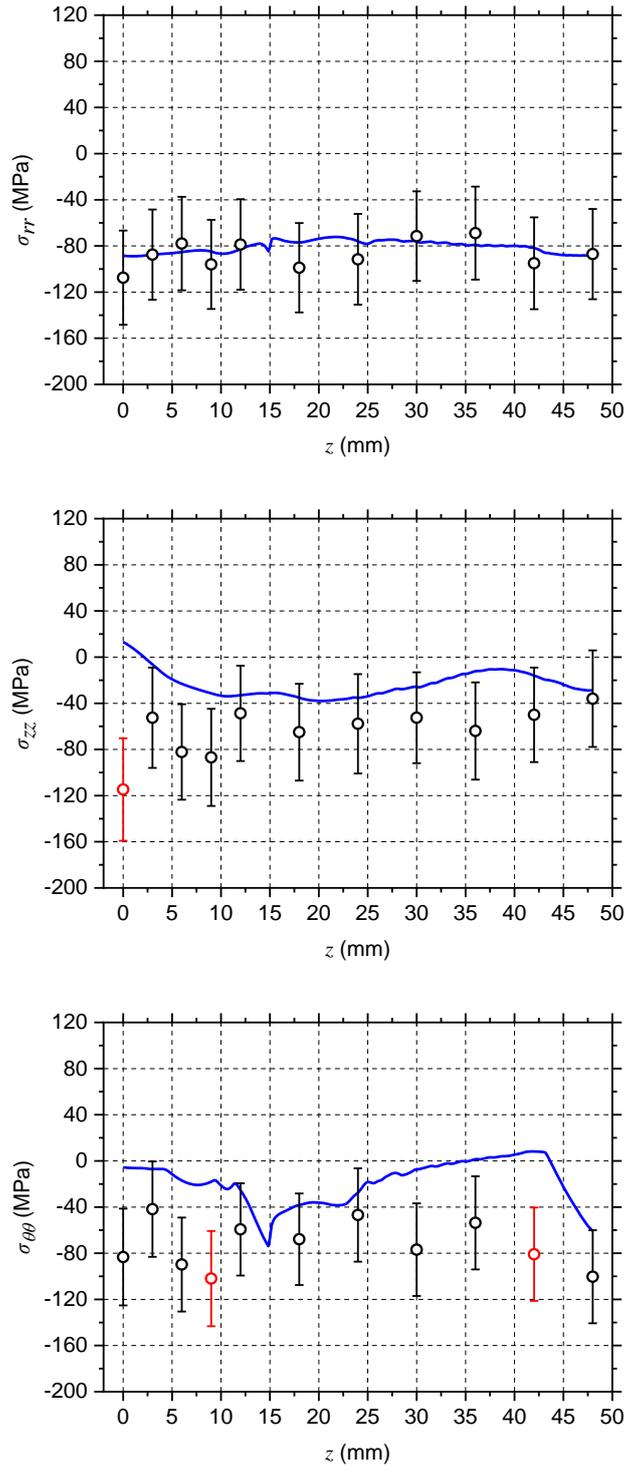
**Fig. 17** Measured (circle marks) vs simulated RS (solid line) as a function of the distance from the joint ( $z$ ) at  $y = -8$  mm for  $\sigma_{rr}$ ,  $\sigma_{zz}$  and  $\sigma_{\theta\theta}$ . The error bars of data points are also shown. Red symbols: positions in which the measured and simulated RS are not in good agreement
