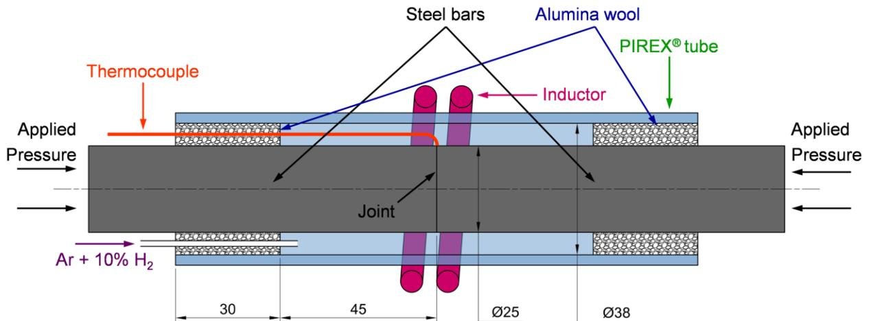
**Fig. 1** Cutaway drawing of the TLPB layout. The relative position of the joint, the steel bars, the inductor of the induction furnace, the thermocouple and the protecting PIREX® tube are indicated. Alumina wool was used as seal between the bars and the protecting tube while the reducing atmosphere was injected through the wool. The applied pressure is indicated and characteristic dimensions in mm are included
