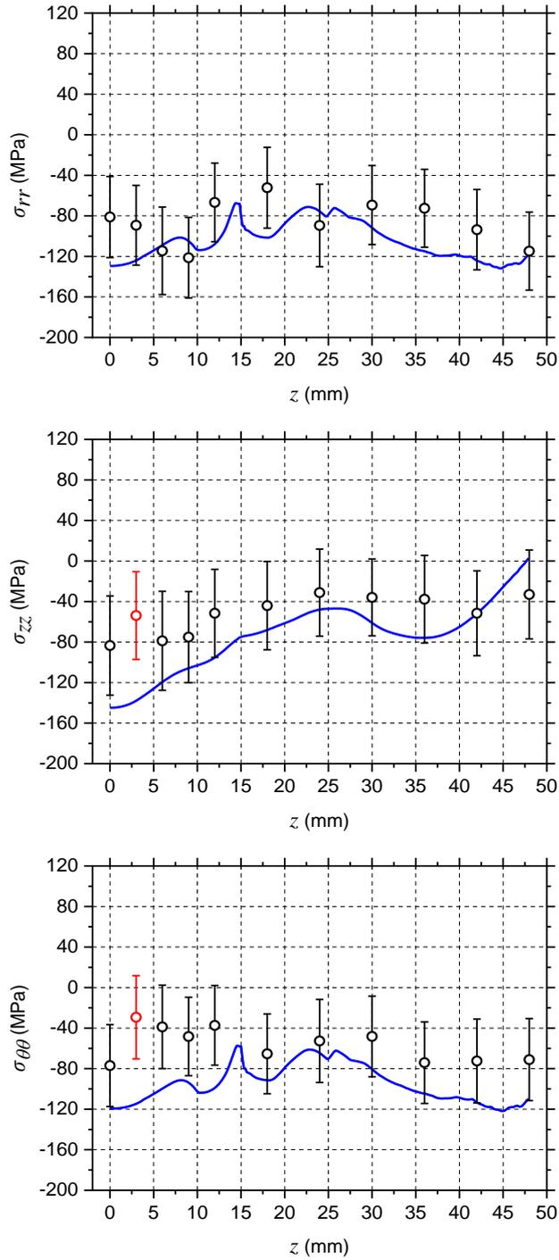
**Fig. 13** Measured (circle marks) vs simulated RS (solid line) as a function of the distance from the joint ( $z$ ) at  $y = 0$  mm for  $\sigma_{rr}$ ,  $\sigma_{zz}$  and  $\sigma_{\theta\theta}$ . The error bars of data points are also shown. Red symbols: positions in which the measured and simulated RS are not in good agreement
