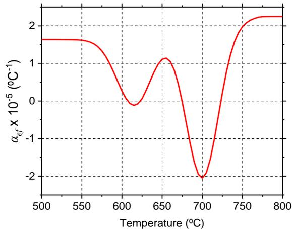
**Fig. 8**  $\alpha_{ef}$  vs temperature during cooling. The dips at 700 and 615 °C are indicating the austenite/ferrite and austenite/pearlite phase transformations, respectively [33]
