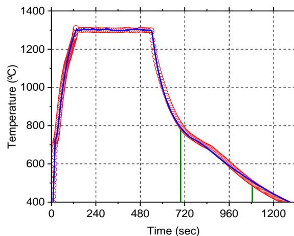
**Fig. 10** Temperature evolution at the joint during TLPB. For the measured data (red circular marks) the elapsed time  $t_{8/5} = 390$  sec is indicated (green solid lines). In
