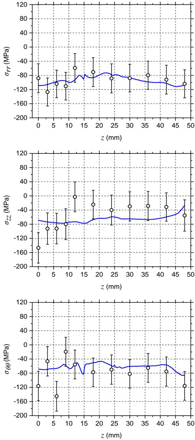
**Fig. 16** Measured (circle marks) vs simulated RS (solid line) as a function of the distance from the joint ( $z$ ) at  $y = -5$  mm for  $\sigma_{rr}$ ,  $\sigma_{zz}$  and  $\sigma_{\theta\theta}$ . The error bars of data points are also shown. At all positions the measured and simulated RS are in good agreement
