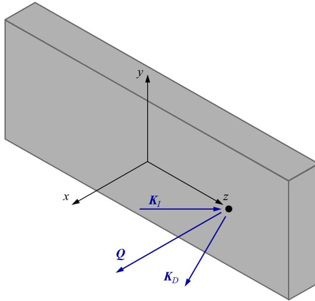
**Fig. 2** Reference sample. Top panel: actual reference sample where the average  $d_0$  vs. distance from the joint ( $z$ ) was measured (the position of the joint is indicated by an arrow mark). Layout to measure  $d_0$  in  $z$  (middle panel) and  $x$  directions (bottom panel). The black point is indicating the centre of a cube, with the corresponding incident beam wavevector ( $K_I$ ), diffracted beam wavevector ( $K_D$ ) and scattering vector ( $Q$ )
