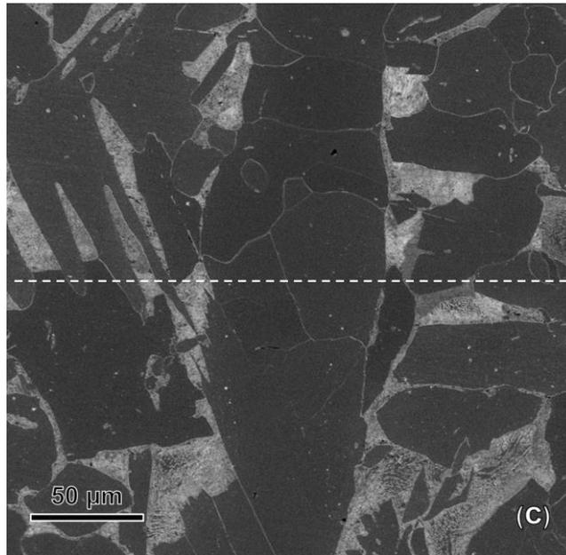
**Fig. 9** Microstructure of the weldment at: the base metal (a), the HAZ (b) and the joint (c). The column of ferrite grains at the joint clearly contrasts with the nearby ferritic/pearlitic microstructure. The  $z$  direction of the weldment (dashed line) is indicated
