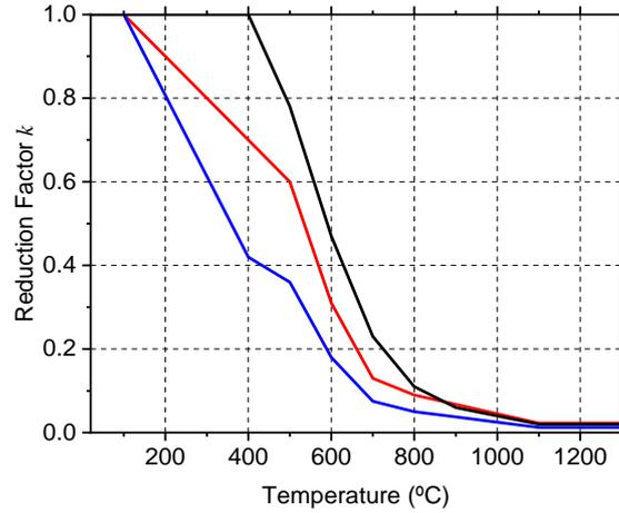
**Fig. 7** Reduction factor  $k$  from ambient to elevated temperature for  $Y$  (red line),  $\sigma_{prop}$  (blue line) and  $\sigma_y$  (black line)
