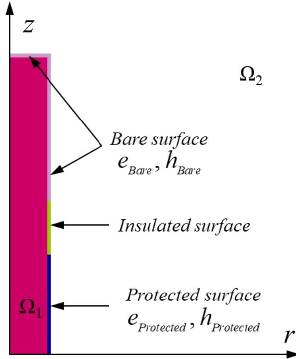
**Fig. 5** Boundary conditions for the thermal analysis. The bare (light violet), insulated (light green) and protected (blue) surfaces are indicated. In addition, the conducting region – the steel bar ( $\Omega_1$ ) – and the nonmagnetic region – the rest of the domain ( $\Omega_2$ ) – are denoted
