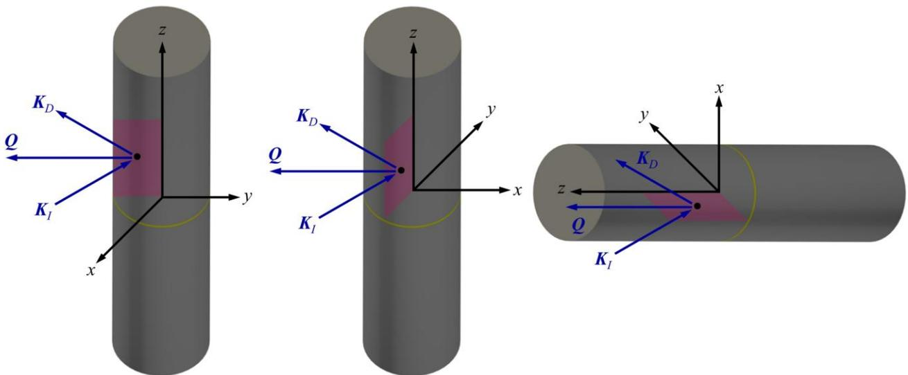
**Fig. 4** Scheme of the strain scanning layout and scanned areas for each measured direction:  $r$  (left),  $\theta$  (centre) and  $z$  (right). Light red areas show the scanned area in each layout (out of scale). Also, the joint position is indicated (yellow line). In each scanned area a point of measurement (black dot) is shown with the corresponding  $K_I$ ,  $K_D$  and  $Q$ .
