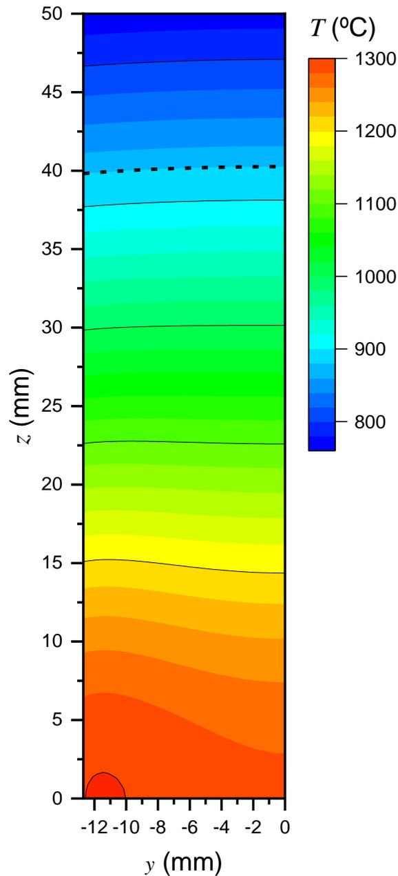
**Fig. 19** Calculated temperature field at the start of the cooling stage in the region where RS were scanned. The dashed line indicates  $A_{C3}$ , showing that up to 40 mm from the joint full austenization was achieved. Partial austenization is achieved for  $z > 40$  mm
