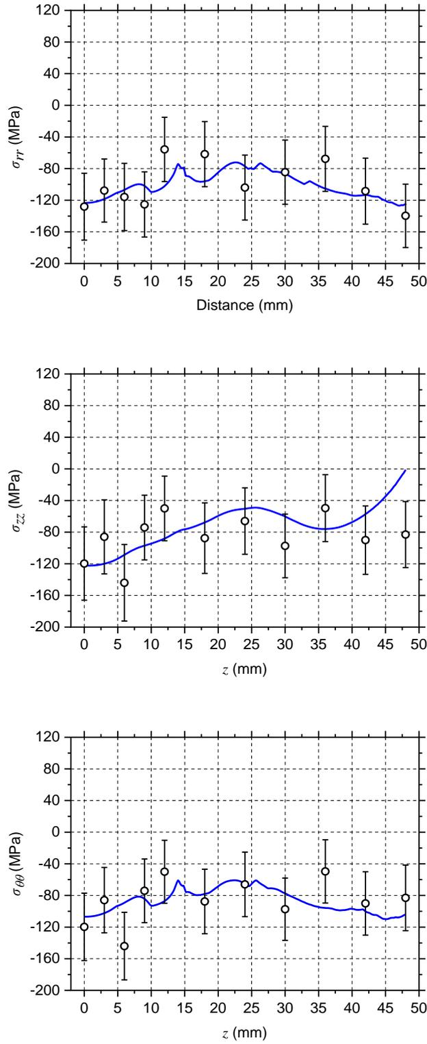
**Fig. 15** Measured (circle marks) vs simulated RS (solid line) as a function of the distance from the joint ( $z$ ) at  $y = -3$  mm for  $\sigma_{rr}$ ,  $\sigma_{zz}$  and  $\sigma_{\theta\theta}$ . The error bars of data points are also shown. At all positions the measured and simulated RS are in good agreement
