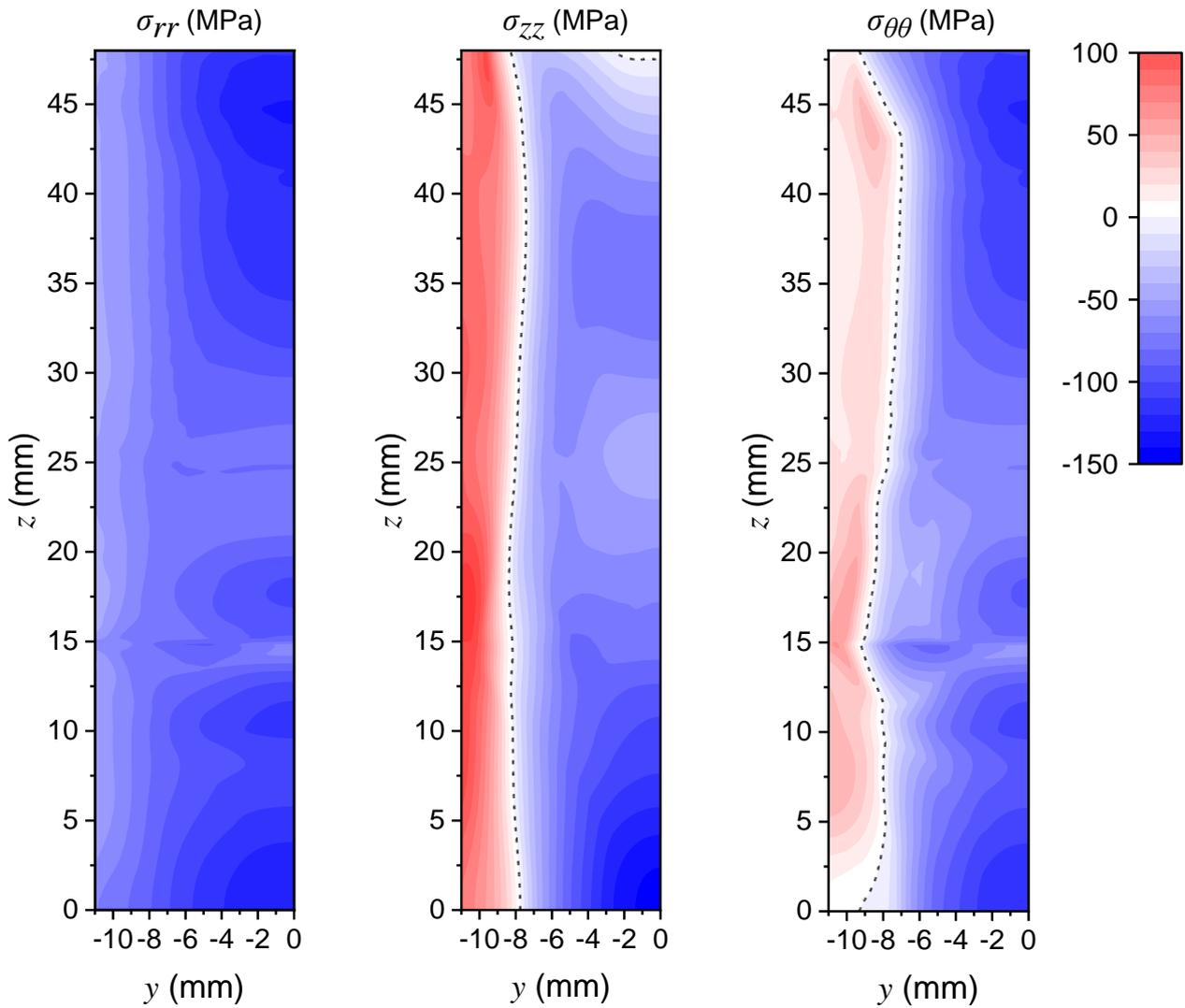
**Fig. 12** Simulated RS at the weldment for  $\sigma_{rr}$ ,  $\sigma_{zz}$ , and  $\sigma_{\theta\theta}$ . Dashed line:  $\sigma_{ii} = 0$  for  $i = r, \theta, z$
