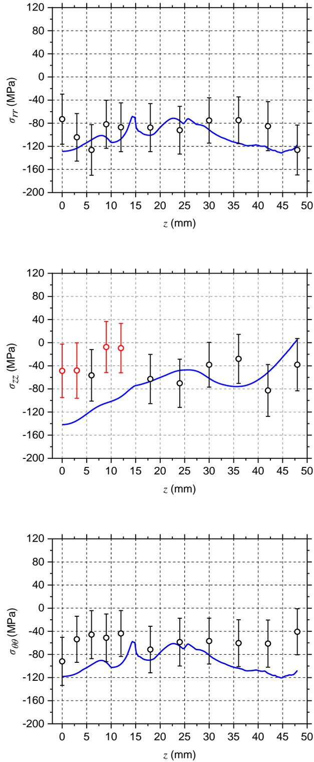
**Fig. 14** Measured (circle marks) vs simulated RS (solid line) as a function of the distance from the joint ( $z$ ) at  $y = -1$  mm for  $\sigma_{rr}$ ,  $\sigma_{zz}$  and  $\sigma_{\theta\theta}$ . The error bars of data points are also shown. Red symbols: positions in which the measured and simulated RS are not in good agreement
