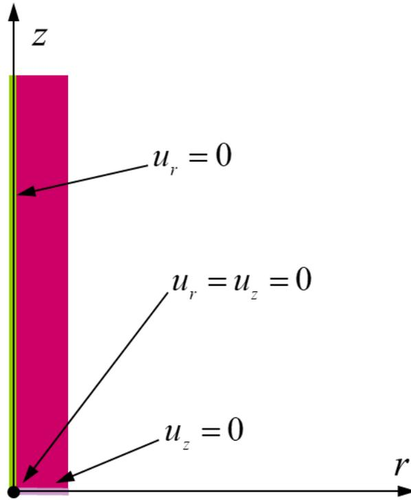
**Fig. 6** Displacement boundary conditions at the weldment. Constraints were applied at the axis of symmetry ( $u_r = 0$ , light green line), at  $z = 0$  ( $u_z = 0$ , light violet line) and at the origin (fixed point, black circle mark)
