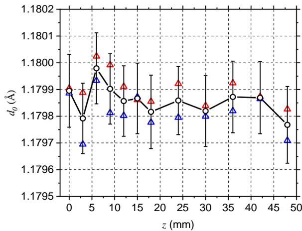
**Fig. 3**  $d_0$  vs distance from the joint ( $z$ ) for the reference sample. Measurements of  $d_0$  in the  $z$  direction (red triangle marks),  $x$  direction (blue triangle marks) and their average
