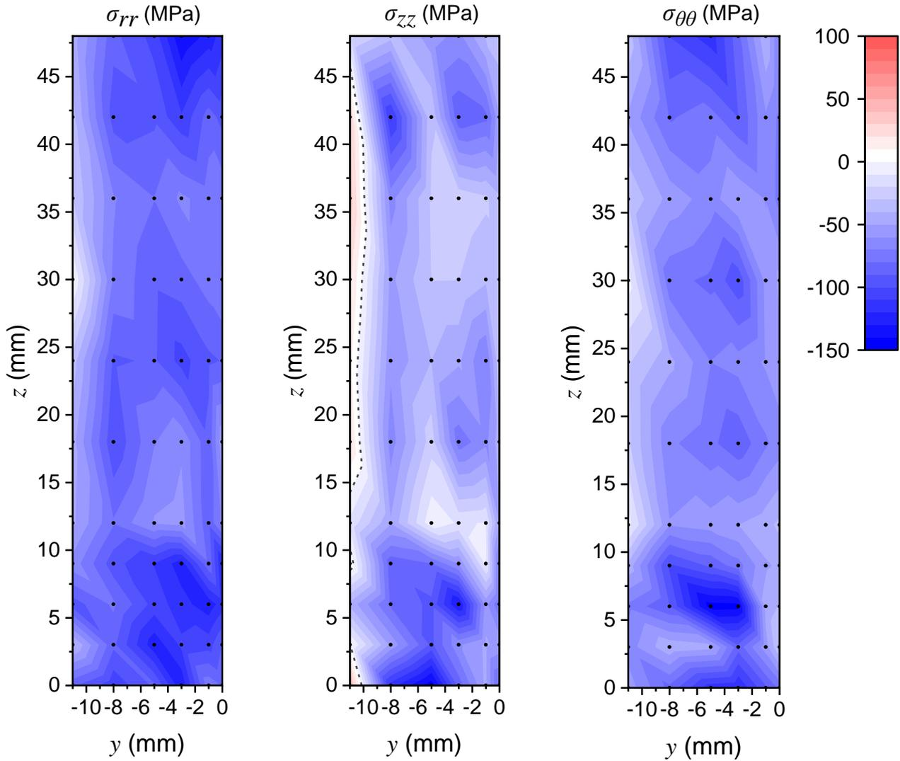
**Fig. 11** Measured RS scanning at the weldment for  $\sigma_{rr}$ ,  $\sigma_{zz}$ , and  $\sigma_{\theta\theta}$ . The measured points are indicated with black dots. Dashed line:  $\sigma_{ii} = 0$  for  $i = r, \theta, z$
