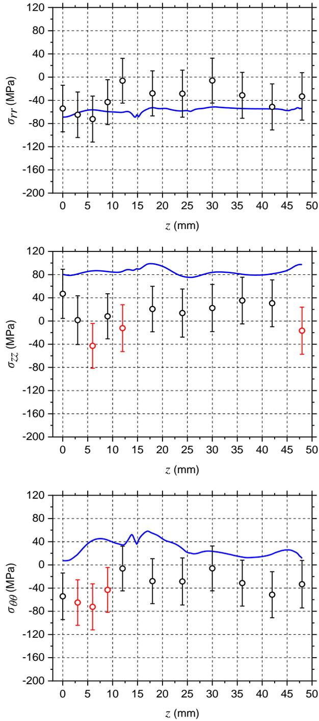
**Fig. 18** Measured (circle marks) vs simulated RS (solid line) as a function of the distance from the joint ( $z$ ) at  $y = -11$  mm for  $\sigma_{rr}$ ,  $\sigma_{zz}$  and  $\sigma_{\theta\theta}$ . The error bars of data points are also shown. Red symbols: positions in which the measured and simulated RS are not in good agreement
