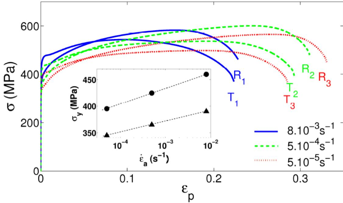
**Fig.1.** True stress versus true strain tensile curves of RD and TD-samples at different initial strain rates. Inset: dependence of the yield stress (measured at  $\epsilon_p = 0.2\%$ ) on the applied strain rate for TD (circles) and RD (triangles) specimens.
