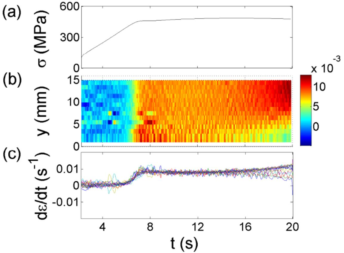
**Fig.4.** (a) Portion of an engineering tensile curve for a TD-specimen deformed at  $\dot{\epsilon}_a = 8 \times 10^{-3} \text{ s}^{-1}$ ; (b) Time–space–local strain rate map obtained using denoising by running average over 100 data points. Some over averaging is used to emphasize the slow global trend. The color bar displays the strain rate scale ( $\text{s}^{-1}$ ); (c) Evolution of the local strain rate for all extensometers.
