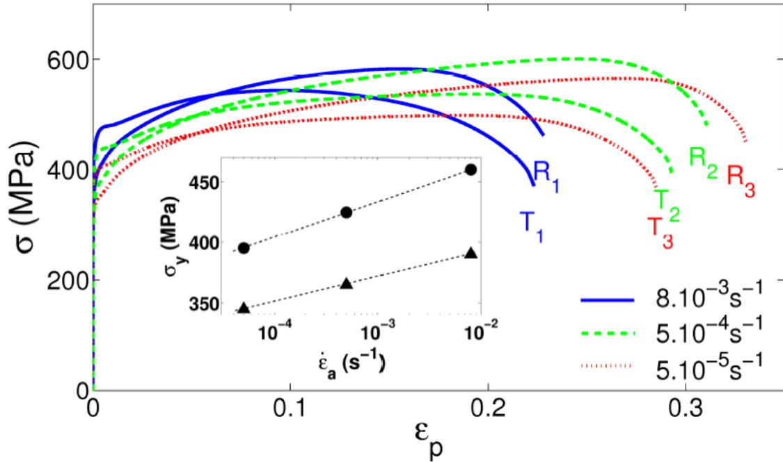
**Fig.1.** True stress versus true strain tensile curves of RD and TD-samples at different initial strain rates. Inset: dependence of the yield stress (measured at  $\epsilon_p = 0.2\%$ ) on the applied strain rate for TD (circles) and RD (triangles) specimens.
