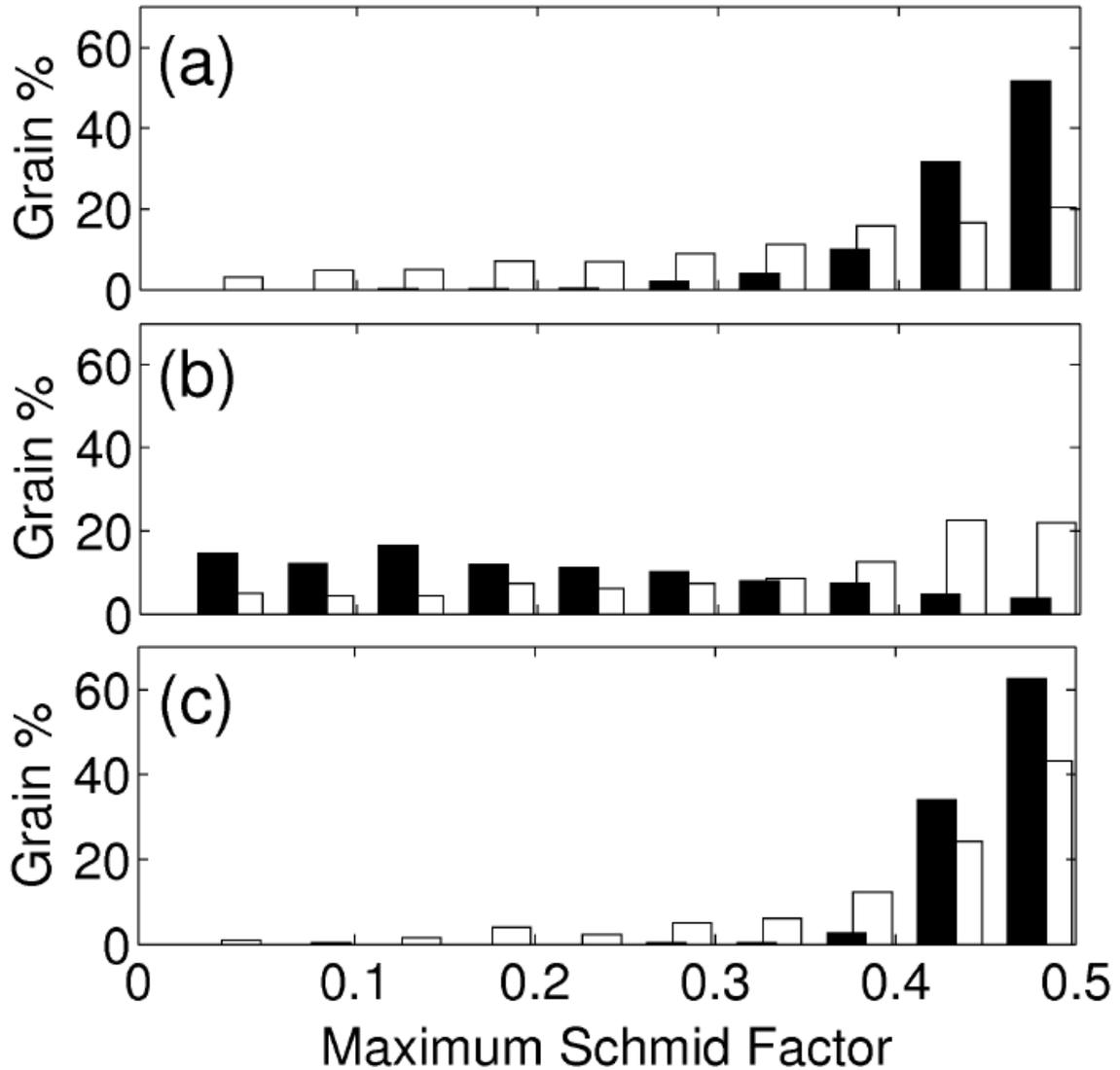
**Fig.2.** Distribution of maximum Schmid factors in grains computed from an EBSD map of an undeformed sample for (a) prismatic, (b) basal, and (c) pyramidal  $\langle a \rangle$  slip systems. Solid bars refer to RD, open bars to TD-samples. The analysis is performed on a  $984 \times 736 \mu\text{m}^2$  area covering more than 600 grains.
