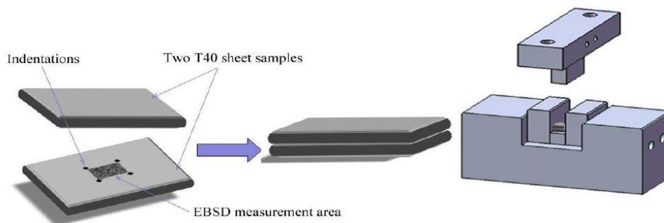
Figure 1: Schematic description of the channel-die set-up used.
