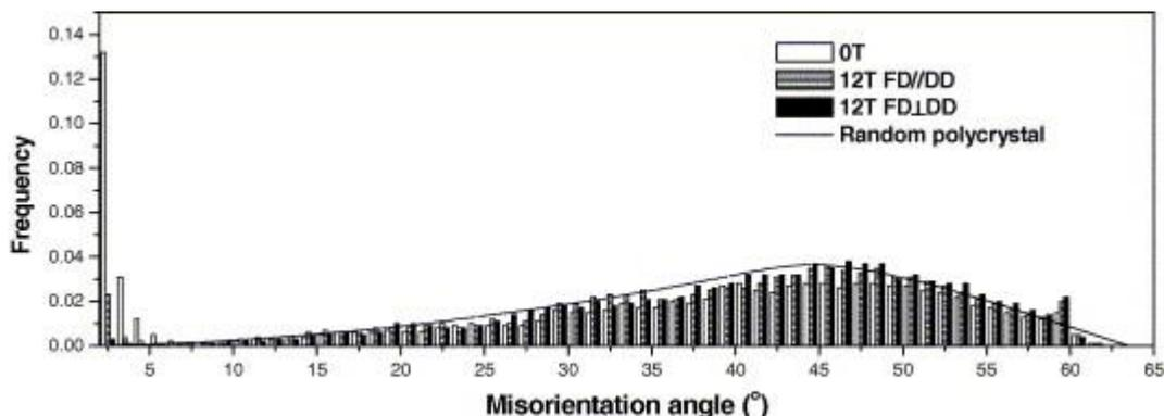
Fig. 2. Misorientation angle distribution of ferrite in specimens austenitized at 870 °C for 10 min and cooled at 23.5 °C/min without and with a 12-T magnetic field.
