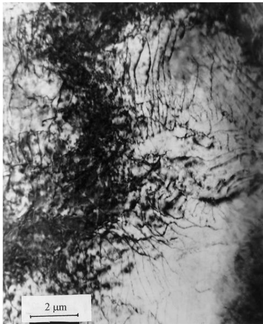
Figure 3 \langle c+a \rangle dislocations on the (2\bar{1}\bar{1}\bar{2}) and (10\bar{1}\bar{1}) planes in a specimen compressed along [0001] (foil normal). Beam direction g = \langle 0002 \rangle .
