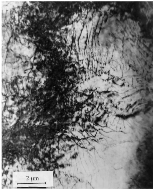
Figure 3 \langle c+a \rangle dislocations on the (2\bar{1}\bar{1}2) and (10\bar{1}\bar{1}) planes in a specimen compressed along [0001] (foil normal). Beam direction g = \langle 0002 \rangle .
