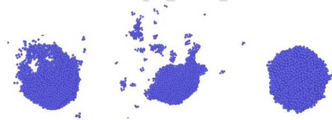
Figure 9- Fourth stage of a 5 nm NP irradiation with a 100 keV PKA. Small fragments are ejected (463 atoms on the initial 4,461 atoms) before the NP annealed itself.
