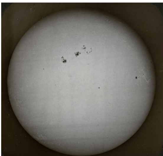
Figure 9: The full Sun observed by Janssen on 2 June 1893 showing sunspot groups and the shutter located at the primary focus of the refractor (at right), allowing extremely short exposure times to freeze the turbulence (courtesy Paris Observatory).
