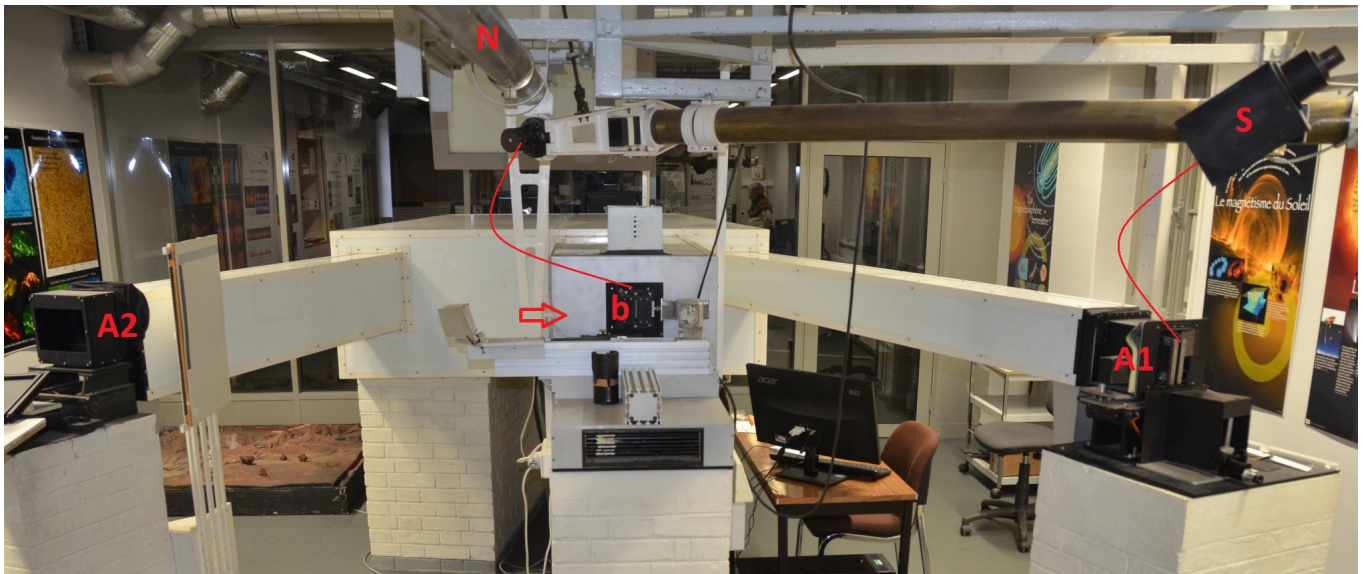
Fig. B.2. Meudon spectroheliograph today. b = entrance slit of the spectrograph ( 30\ \mu\text{m} width). A1 and A2 are old photographic arms (chambers not used any more). N is the mechanical coupling between the entrance objective (a) of Figure B.1 and the moving artificial moon (a round neutral density 1 of 37 mm diameter). This attenuator is located in the image plane and avoids the saturation of the disk in the case of prominence observations with long exposure time. S is an old visual flare spectrohelioscope (no more used), composed of a high speed rotating prism which translates active region images upon the slit ( b ), and an ocular (S) to observe the the wavelength selected by the output slit located in A1.
