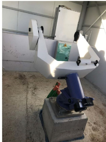
Fig. 2 The MTSP housing. Left: the MTSP building at Calern observatory (1270 m, Côte d'Azur). It moves on two rails and is computer controlled. It is closed by metallic curtains and connected to many environment detectors (such as cameras and meteorological devices) for automatic operation. Right: the equatorial mount waiting for the instruments.
