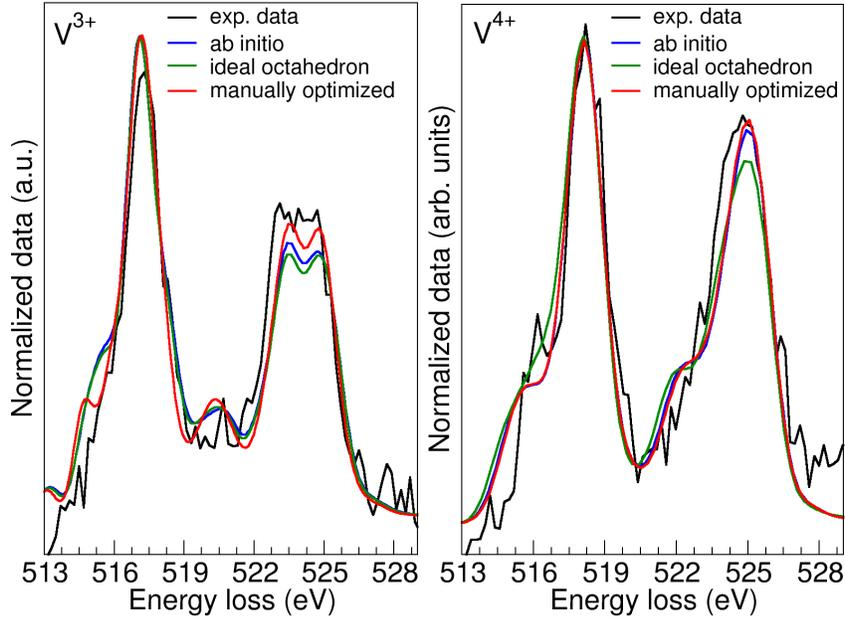
Figure 5: Simulation of  $V^{3+}$  and  $V^{4+}$  XRS spectra with Hilbert++ and optimal empirical parameters considering a distorted octahedron given by *ab initio* optimisation (blue line), an ideal octahedron (green line), and finally a distorted octahedron whose coordinates have been manually optimised (red line).
