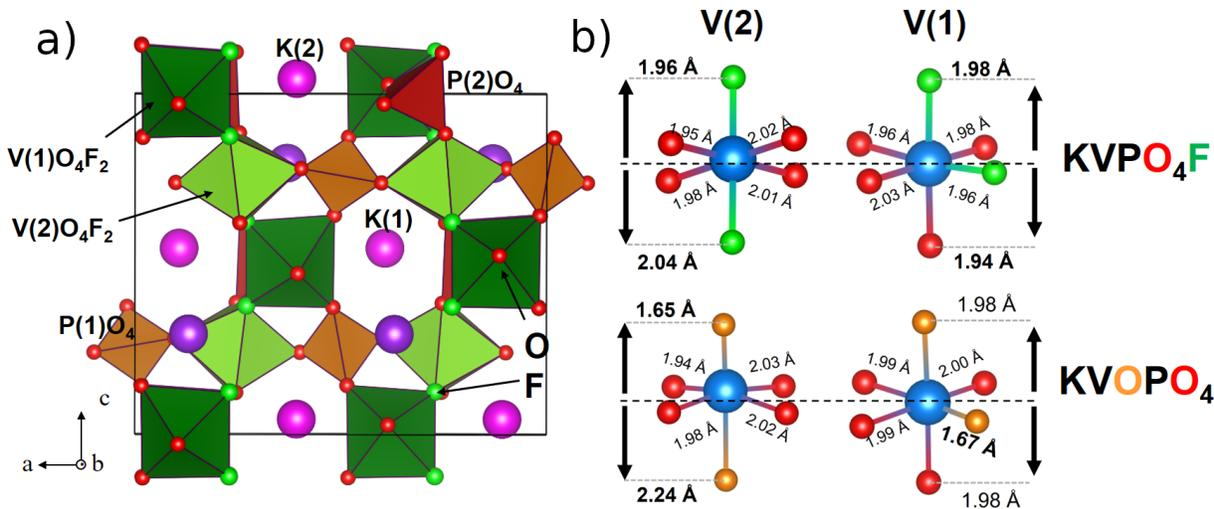
Figure 1: a) Crystal structure of  $\text{KVPO}_4\text{F}$ . The F sites can be completely or partially substituted by oxygen, up to the composition  $\text{KVOPO}_4$ . b) Detailed experimental bond length of the first coordination shell in  $\text{KVPO}_4\text{F}$  (top) and  $\text{KVOPO}_4$  (bottom) for both vanadium sites.
