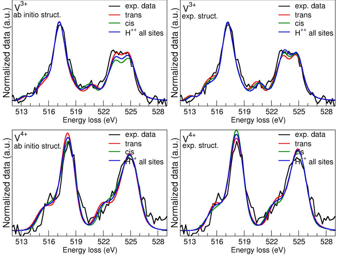
Figure 4: Energy loss spectra for  $\text{KVPO}_4\text{F}$  and  $\text{KVOPO}_4$  systems. The corresponding  $\text{V}^{3+}$  and  $\text{V}^{4+}$  spectra are calculated on the basis of the Wannier Hamiltonian for the *ab initio* structures (left panel) and experimental structures (right panel).
