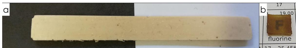
Figure 3. a. Crosslinked material after 8 h at room temperature (ca.  $20\text{ }^{\circ}\text{C}$ ); and b. after 3 h at  $150\text{ }^{\circ}\text{C}$
