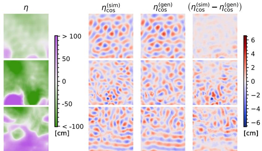
**Figure 2.** A few examples of individual tests. Top row: snapshot with the highest correlation among all sets (belongs to ET1). Middle and bottom rows: same for the lowest correlations among ET1–ET4, and ET1–ET5, respectively (belong to ET4 and ET5, respectively). For legibility, we omit spatial axis labels, noting that the first, second, and third rows correspond to down-jet, down-jet, and mid-jet bands, respectively; see Figure 1 for their definitions.
