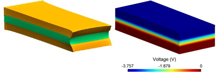
Fig. 5. Amplified displacement field and nodal voltage (V).
