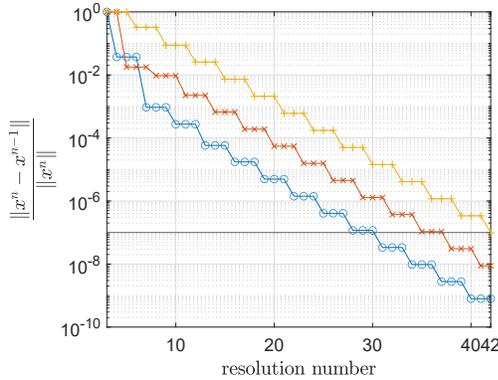
Fig. 7. Convergence ratio of magnetic (o), mechanical (x) and electric (+) solutions after given  $n^\circ$  of resolutions for the block Gauss-Seidel algorithm with a 1-2-3-1... resolution pattern for the given mesh.  $\|x^n\|$  Relates the  $n$ th solution of the given problem.
