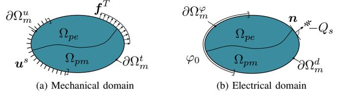
Fig. 2. Mechanical and electrical domains. With  $\mathbf{f}^T$  the surface forces,  $\mathbf{u}^s$  the imposed displacement,  $\varphi_0$  the imposed electric potential and  $Q^s$  the surface charge density.
