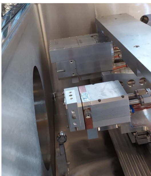
Figure 3. Pictures of the internal mechanics showing the old CCD (front) and the new CMOS (back) detectors installed on their internal carriages, and of the MCP-DL detector. Each detector can be positioned on the x-ray beam axis and the displaced along it with a travel of 52 cm, in order to adjust the sample-detector distance.
