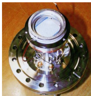
Figure 3. Pictures of the internal mechanics showing the old CCD (front) and the new CMOS (back) detectors installed on their internal carriages, and of the MCP-DL detector. Each detector can be positioned on the x-ray beam axis and the displaced along it with a travel of 52 cm, in order to adjust the sample-detector distance.
