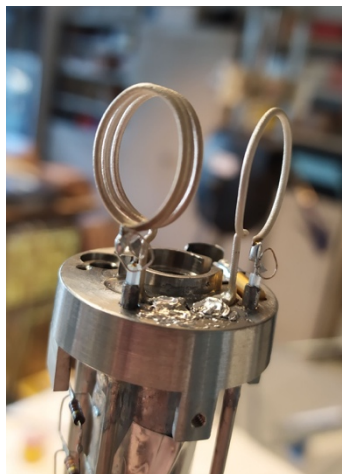
Figure 13: Photograph of the perpendicular coupling coils used for inductive detection attached to co-axial transmission cables. The ^1\text{H} channel uses a single loop, whilst the ^{13}\text{C} channel employs three tightly wound loops of smaller diameter. This structure is housed within a brass “cap” whilst in liquid helium. The choice of a cylindrical rf -coil support is necessary to accommodate the sample dissolution stick and to fit into the bore of the polarizer. The two rf -coil loops are elliptical loops of 12 \times 16 mm in diameter.
