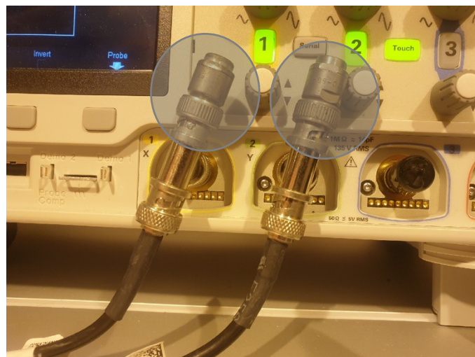
Figure 19: Photograph of 50 \Omega resistors (grey shading) used to protect the oscilloscope whilst performing rf -coil cross-talk characterizations.
