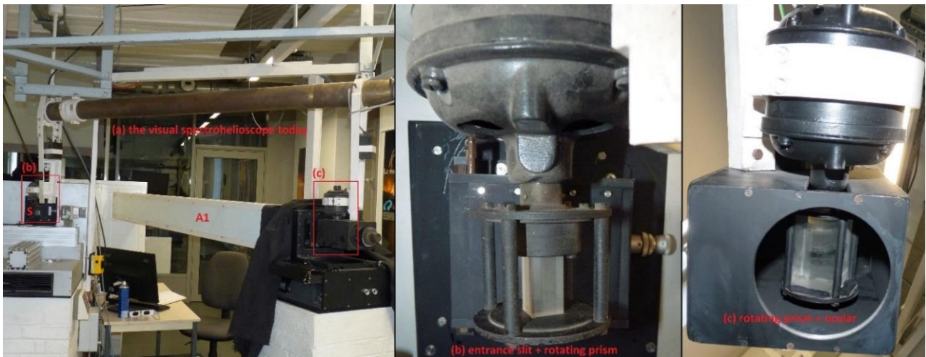
Figure 39. (a): the visual spectroheliograph worked with two high speed rotating prisms, respectively at the entrance slit (b box) and at the output slit (c box) in the spectrum. Two synchronous motors replaced the single motor of Figure 38, so that the complex mechanics was removed. (b): the prism (14 mm square section) in the image plane (motor above). (c): the prism (32 mm square section) in the spectrum between the exit slit and the ocular (motor above). The section ratio (32/14) corresponds to the spectrograph magnification (2.31). Courtesy Paris Observatory.
