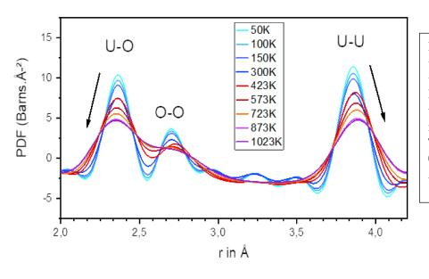
Neutron PDF(r) results from 50 to 1023 K. The r(U-U) follows the thermal expansion, as it must. However, the r(U-O) *decreases* with increasing temperature as a result of the phonon correlations The r-space resolution is about 0.16 Å (FWHM) for a  $Q_{max} = 23.5$  Å<sup>-1</sup>. Taken from Ref. [1]
