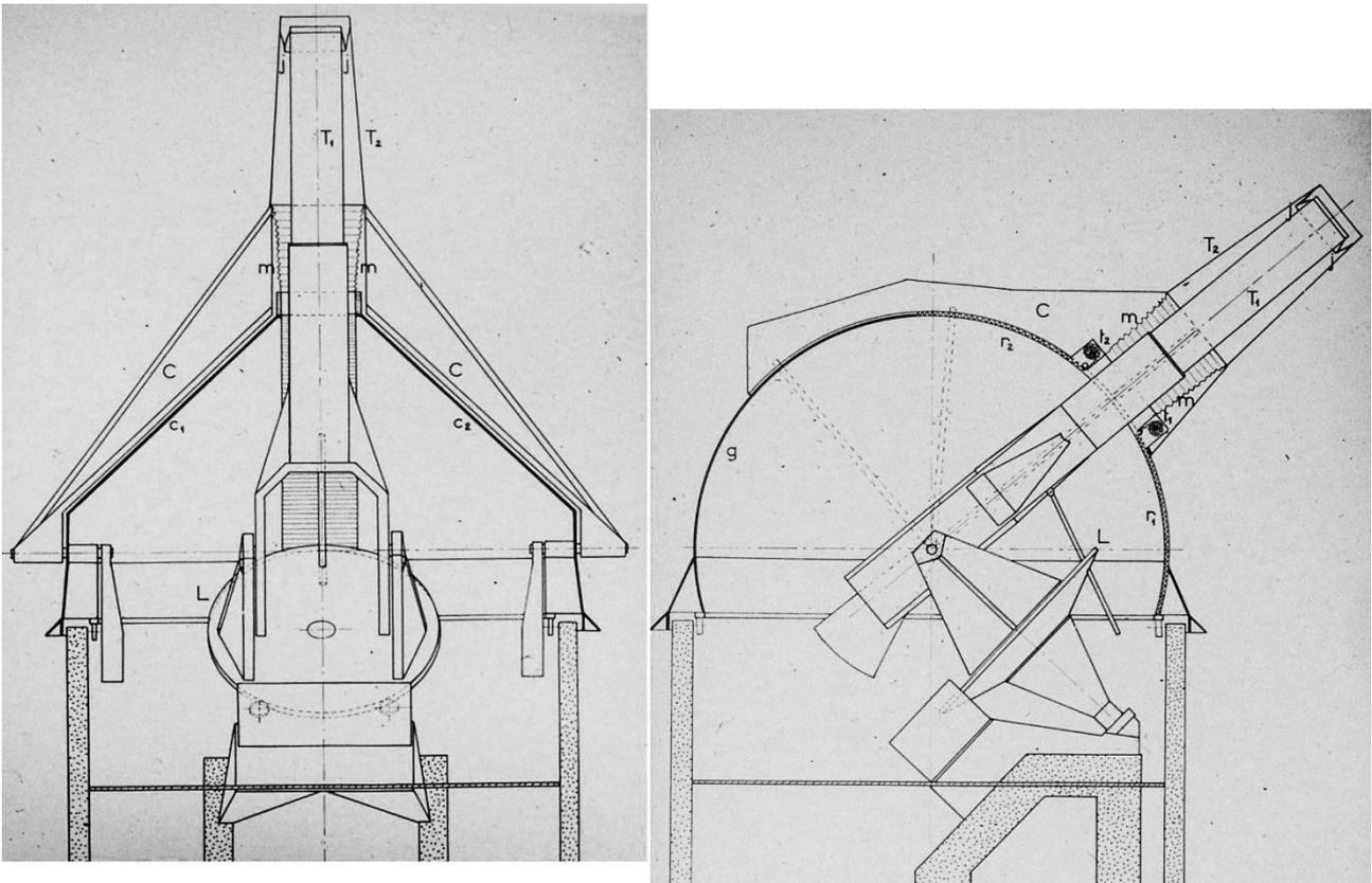
Figure 3: Drawings of the Turret-Dome (1960). C, c<sub>1</sub>, c<sub>2</sub>, T<sub>2</sub> = helmet structure; g = dome; T<sub>1</sub> = refractor tube; j, m = flexible washers; r<sub>1</sub>, r<sub>2</sub> = rolling curtains; L = equatorial table and fork (courtesy OMP).
