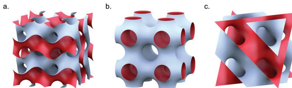
**Figure 2.** Examples of three triply periodic minimal surfaces. a) Gyroid, b) primitive cubic surface, and c) diamond cubic surface. Adapted with permission.<sup>[16]</sup> Copyright 2014, Walter de Gruyter Berlin/Boston.
