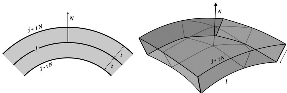
**Figure 1.** Illustration of the Steiner Offset for a line segment (left) and a surface patch (right). Adapted with permission.<sup>[13]</sup> Copyright 2019, The Author.
