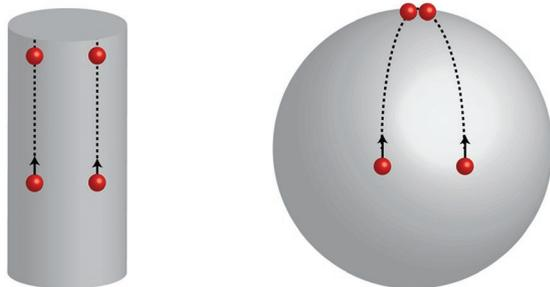
**Figure 4.** A cylinder and a sphere have, respectively, zero and nonzero positive Gaussian curvatures. Two particles moving parallel to each other on a cylinder (zero Gaussian curvature surface) will never collide. However, particles moving parallel to each other on a nonzero Gaussian surface (e.g., sphere) will converge (or diverge for negative Gaussian curvature surfaces).
