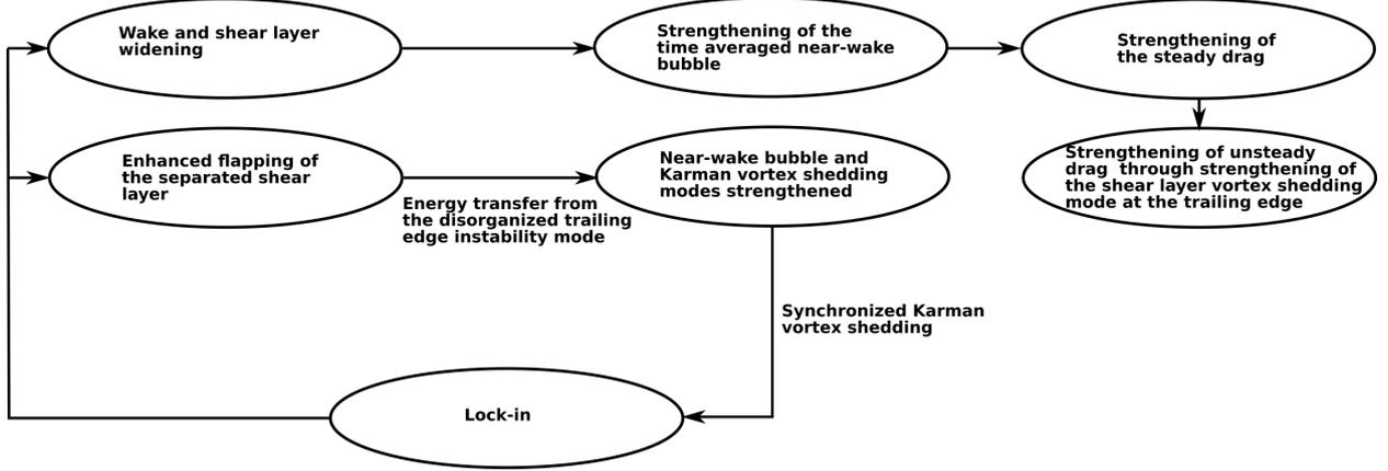
Figure 35: Conceptual sketch of energy transfer at lock-in with the twisting mode of a blunt plate with chord to thickness ratio  $c/D = 16$ .
