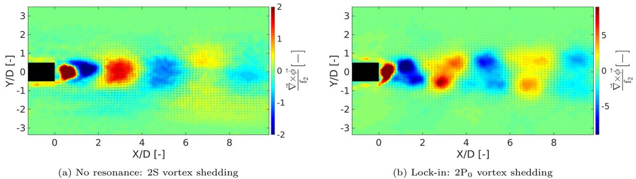
Figure 33: Snapshot of the (x,y) cartography of the reconstructed vorticity, including modes 1 to 9 at (a) the non resonance regime ( $Re_c = 3.0 \times 10^5$ ) and (b) the lock-in regime ( $Re_c = 5.7 \times 10^5$ ).
