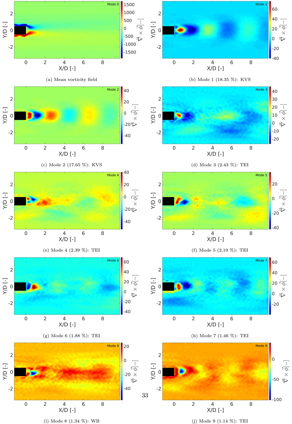
Figure 28: (x,y) cartography of vorticity. Mean vorticity field and spatial POD modes from 1 to 9 at  $U_0 = 3.0 \text{ m.s}^{-1}$ .
