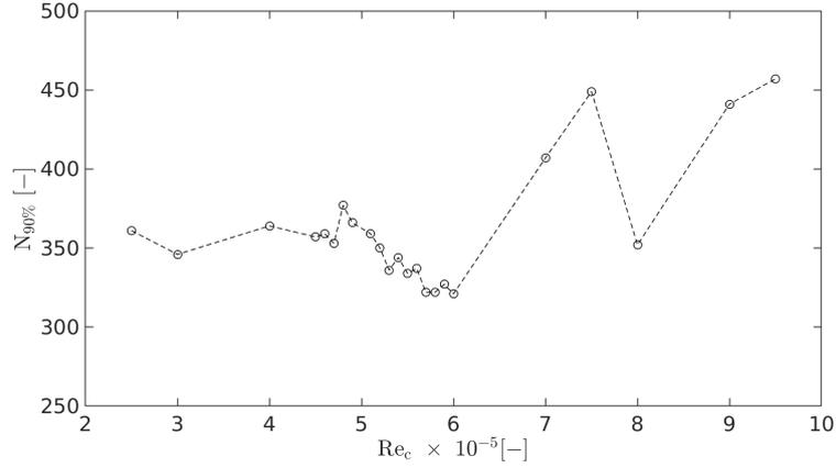
Figure 25: Number of modes to reach 90% of the total energy according to Reynolds number.
