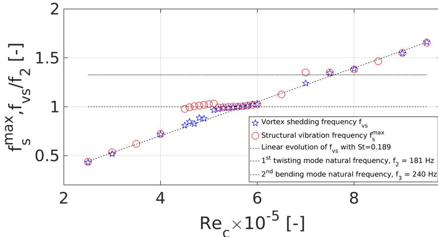
Figure 10: Evolution with Reynolds of the structural vibration frequency  $f_s^{\max}$  and Karman vortex shedding frequency  $f_{vs}$  scaled by  $f_2$ . Maximal uncertainty is 0.6 Hz for  $f_s^{\max}$  and 1 Hz for  $f_{vs}$ .
