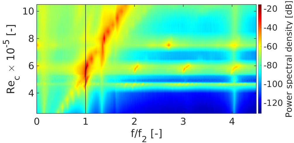
Figure 11: Cartography of the power spectral density of the structure vibration velocity. Cartography in the plane  $(f_s/f_2, Re_c)$ . Power spectral density expressed in dB ( $V_{s,ref} = 1 \text{ m.s}^{-1}$ ). Figure extracted from our ASME paper, Watine et al. (2020) [21].
