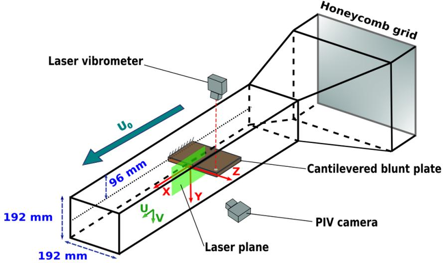
Figure 1: Test section of the IRENav hydrodynamic tunnel.
