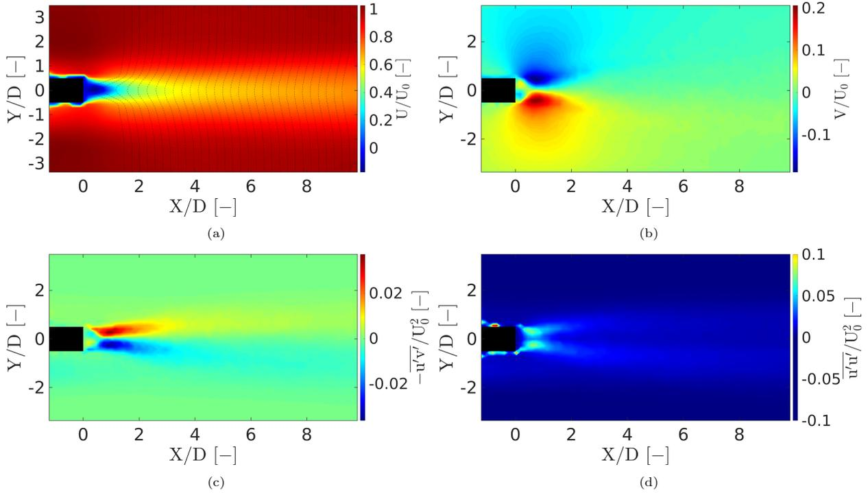
Figure 13:  $(x,y)$  cartography of the time averaged horizontal (a) and vertical (b) velocity components  $U$  and  $V$ , the Reynolds shear stress  $-\overline{u'v'}/U_0^2$  (c) and the Reynolds normal streamwise stress  $\overline{u'u'}/U_0^2$  (d) at  $U_0 = 3.0 \text{ m.s}^{-1}$ . Cartographies based on the reconstructed velocity field.
