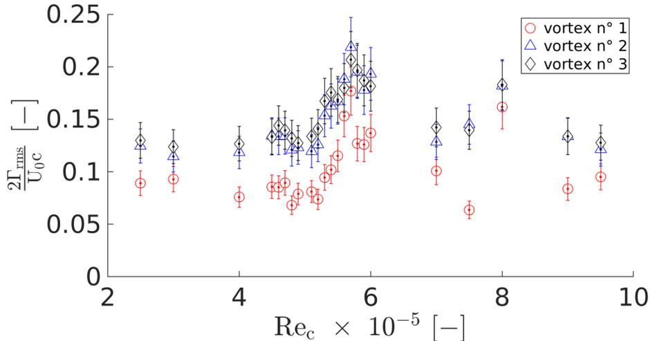
Figure 24: Mode 1 rms circulation evolution with Reynolds of the three first vortices downstream of the trailing edge (mode 1). The circulation is scaled by  $\frac{U_0 c}{2}$ , which is representative of the lift coefficient. Vortex 1 is the upstream vortex, vortex 3 is the downstream vortex.
