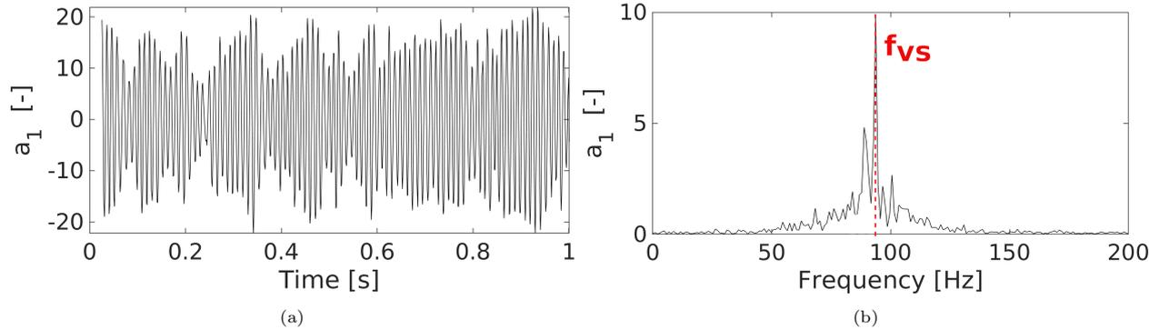
Figure 8: Time evolution (a) and associated frequency spectrum (b) of the POD coefficient  $a_1(t)$ , characteristic of the Karman wake at  $U_0 = 3.0 \text{ m.s}^{-1}$ . The Karman vortex shedding frequency is expressed as  $f_{vs}$  and corresponds to the highest peak of the spectrum.
