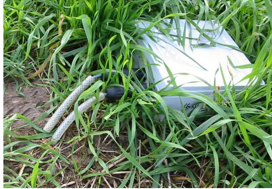
**Figure 1.** One-channel sensor of last generation during a field trial. Box containing electronics, and aerial part of lead towards electrodes in the soil.
