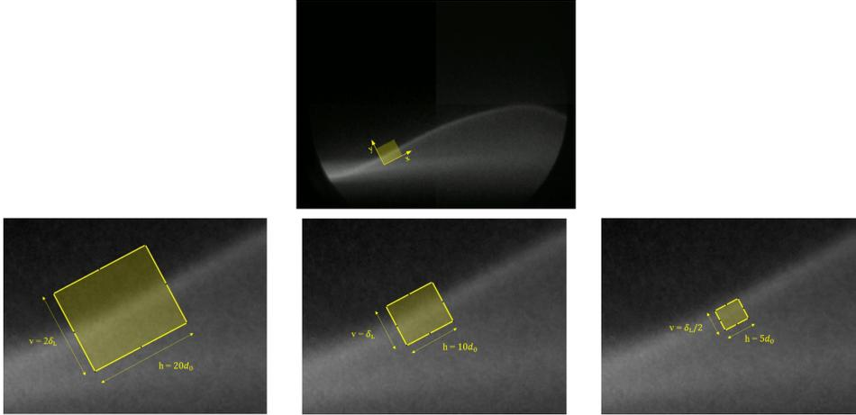
**Figure 4.** Chemiluminescence image of  $\text{C}_3\text{H}_8/\text{air}$  flame at  $\phi = 1.3$  with the region of interest (yellow) having different sizes depending on the flame thickness and initial droplet size
