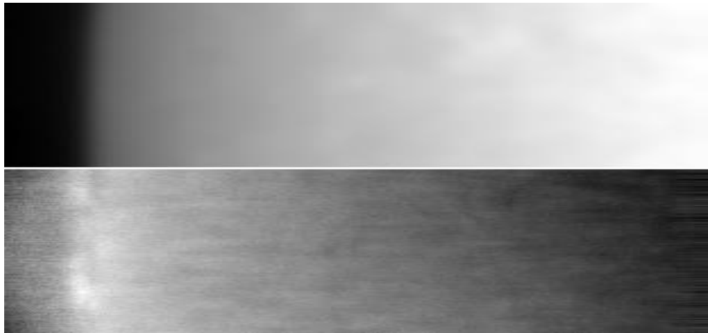
Figure 19 : Polarization of the continuum at 393 nm through a 10 nm filter in imagery mode. Top: intensity I . Bottom: polarization rate Q/I . Courtesy Paris observatory.
