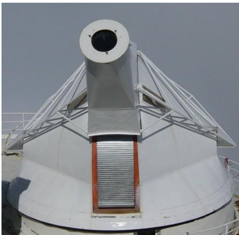
Figure 1 : The tube of the 50 cm/6.45 m refractor of the Pic du Midi Turret Dome (2870 m elevation). Mehlretter's ring is mounted during observations to avoid the heating of the lens holder. The dome is closed by moving curtains. Courtesy Observatoire Midi Pyrénées (OMP).
