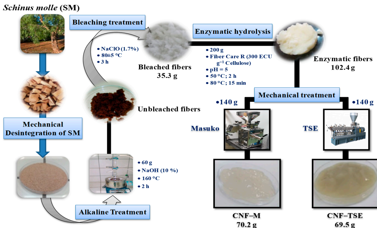
Figure 1. Schematic illustration of procedures used to produce CNF from Schinus molle .
