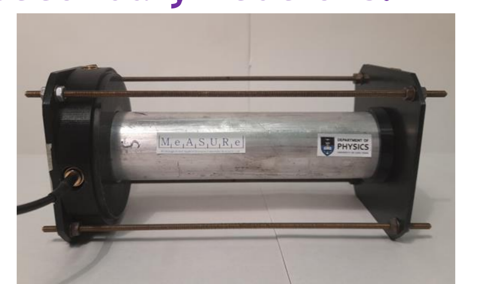
Figure 9. Prototype of the compact neutron detector based on scintillator from MeASURE.
