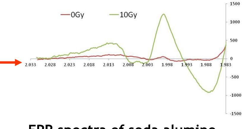
EPR spectra of soda alumino silicate glass
