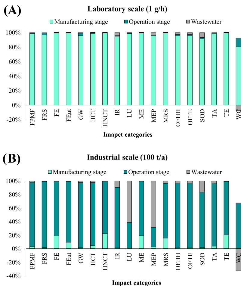
Figure 6. Total contribution of each impact for the manufacturing stage, operation stage, and wastewater at (A) laboratory scale and (B) industrial scale.
