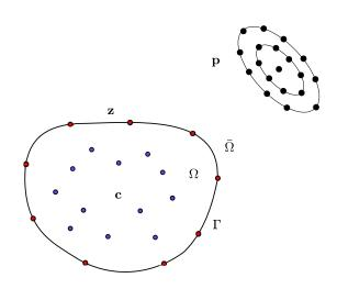
FIG. 1. (Color online) A set of equivalent monopolar sources with complex amplitudes  $\mathbf{c}$  (blue dots) is sought after to match both the impedance condition  $\mathbf{z}$  on the skin of the body and the pressure  $\mathbf{p}$  measured by a microphone array at a given frequency.
