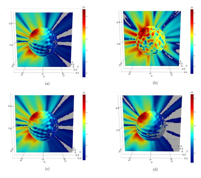
FIG. 5. (Color online) Acoustic pressure (amplitude) on  $\Gamma_{\rm obs}$  radiated by 5 randomly correlated monopoles at ka=13 (with a 20 dB dynamic range). (a) Analytical sound field. (b) Sound field propagated by sources identified with iBF featuring free-field FRF. (c) Sound field propagated by sources identified with iBF featuring analytical FRF. (d) Sound field propagated by sources identified with Galerkin ESM.
