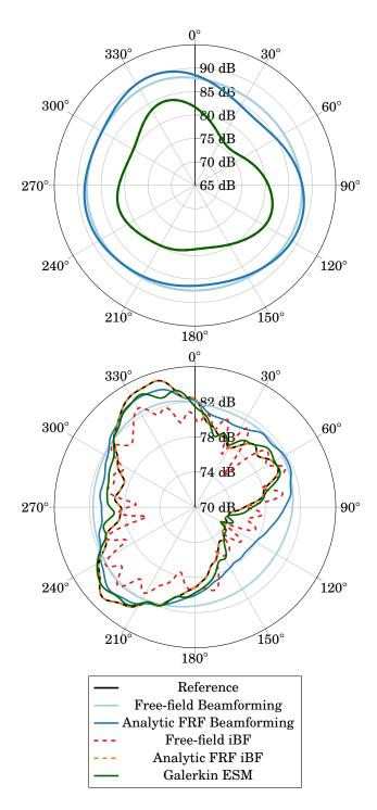
FIG. 3. (Color online) Directivity pattern of 10 uncorrelated monopoles on a rigid sphere at ka=1 (top) and ka=13 (bottom), computed through various imaging algorithms. At low frequency, both Galerkin ESM and iBF are matching with the reference (all 4 plots are overlapped).
