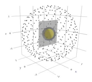
FIG. 2. (Color online) Geometrical set-up for validation. The yellow surface is the control point support  $\Gamma$ , the transparent grey is  $\Gamma_{\rm obs}$  and the cloud of points around it is the microphone array.
