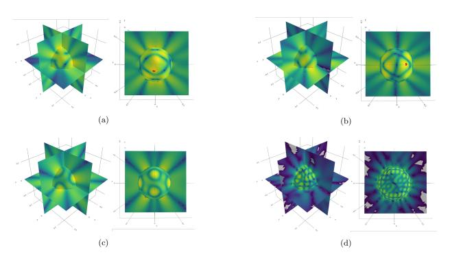
FIG. 7. (Color online) Pressure amplitudes on  $\Gamma_{\rm obs}$  radiated by the  $i^{\rm th}$  column of  $\mathbf{Q}_2\mathbf{\Lambda}$  ( $\mathbf{\Lambda}$  being defined by Eq.(17)). (a) i=1, (b) i=10, (c) i=100, (d) i=250 and ka=8.24. Plots are displayed within a 30 dB dynamic range, and the red dot indicates the maximum level location.
