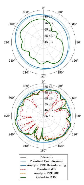
FIG. 4. (Color online) Directivity pattern of 10 correlated monopoles on a rigid sphere at ka=1 (top) and ka=13 (bottom), computed through various imaging algorithms. At low frequency, both Galerkin ESM and iBF are matching with the reference (all 4 plots are overlapped).
