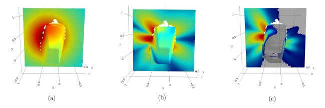
FIG. 11. (Color online) Acoustic pressure (amplitude) backpropagated on  $\Gamma_{\rm obs}$  at kL=21 (relative levels with a 30 dB dynamic range). (a) Sound field propagated by sources identified with CBF featuring free field FRF. (b) Sound field propagated by sources identified with iBF featuring free field FRF. (c) Sound field propagated by sources identified with Galerkin ESM.
