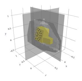
FIG. 10. (Color online) Numerical set-up for experimental set up. The yellow surface is the control point support  $\Gamma$ , the transparent grey is  $\Gamma_{\rm obs}$  and the 36 black dots represent the microphone array placed at 12 cm from the mock-up.
