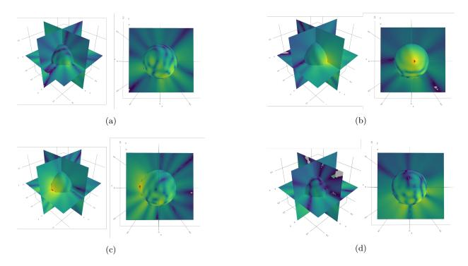
FIG. 6. (Color online) Pressure amplitudes on  $\Gamma_{\rm obs}$  radiated by the  $i^{\rm th}$  column of  ${\bf Q}_2{\bf \Lambda}$  ( ${\bf \Lambda}$  being the identity matrix). (a) i=1, (b) i=10, (c) i=100, (d) i=250 and ka=8.24. Plots are displayed within a 30 dB dynamic range, and the red dot indicates the maximum level location.
