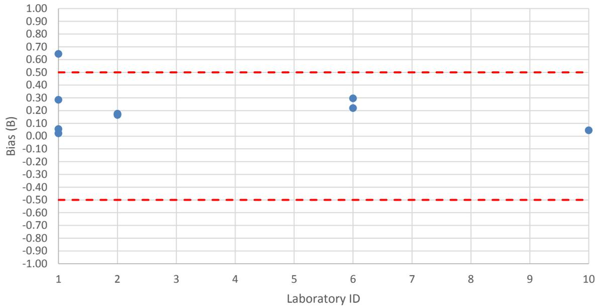
Figure 13. Biological neutron dosimetry performance for Irradiation #1.
