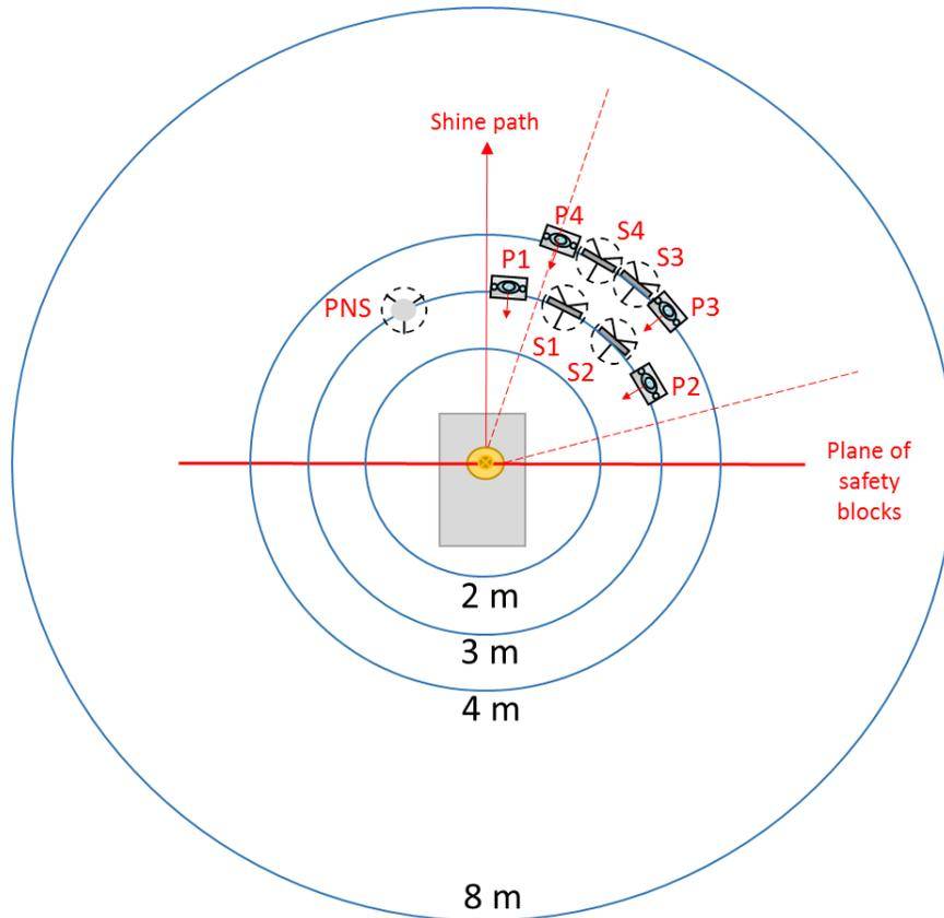
Figure 1: Location of dosimetry phantoms (P#) and stands (S#) for irradiation 1.
