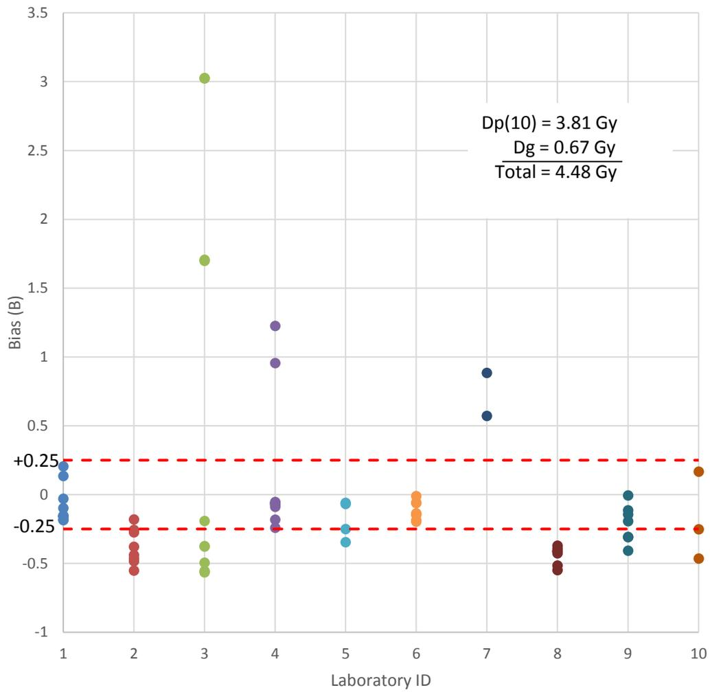
Figure 5. Irradiation No.2 - Comparison of final total dose results to ANSI 13.3 Limits @ 3m
