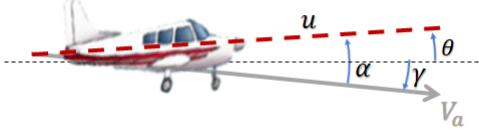
Fig. 2: Representation of the aircraft angles in the vertical plane for a descending flight.
