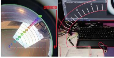
Fig. 3. Right: Photo of a protractor with red dots denominated real elevation overlaid with elevation estimated by the program. Left: overview of the test setup.
