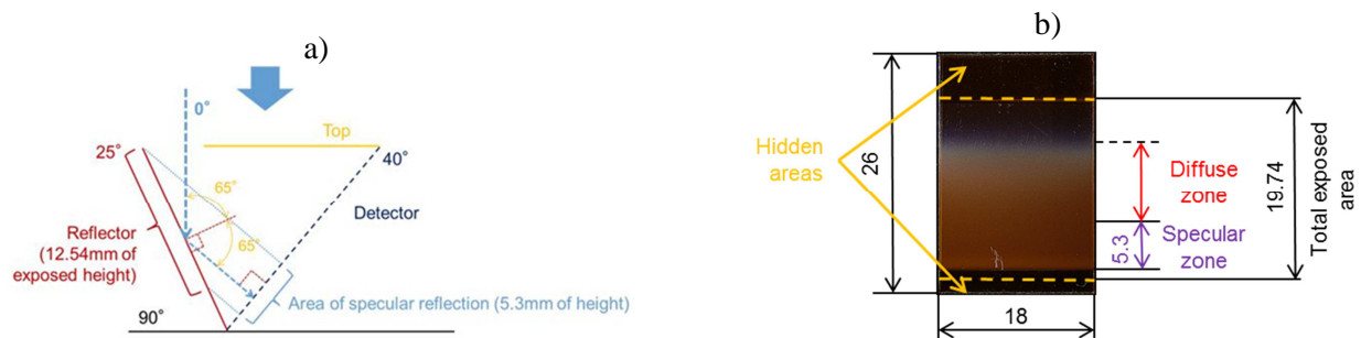
Figure 4. a. Reflection angles inside a geometry. b. Optical observation of erosion areas for PCC sample.
