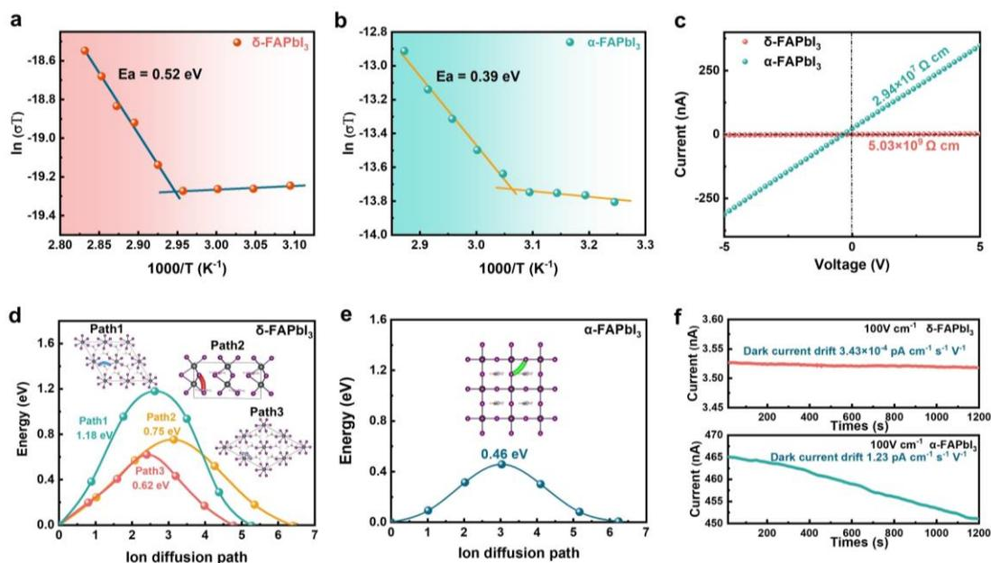
**Figure 3.** Ionic migration in  $\delta$ -FAPbI<sub>3</sub> and  $\alpha$ -FAPbI<sub>3</sub>. Temperature-dependent conductivity of the (a)  $\delta$ -FAPbI<sub>3</sub> wafer and (b)  $\alpha$ -FAPbI<sub>3</sub> wafer. (c) The resistivity of  $\delta$ -FAPbI<sub>3</sub> and  $\alpha$ -FAPbI<sub>3</sub> wafers.
