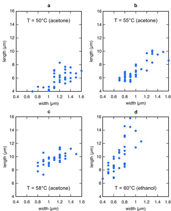
**Figure 3.** Length and width of a population of single crystals prepared from fraction SAA14–21 (0.05% w/v) at different temperatures by diffusion of acetone (a-c) or ethanol (d) vapors. The dimensions have been measured from SEM images.
