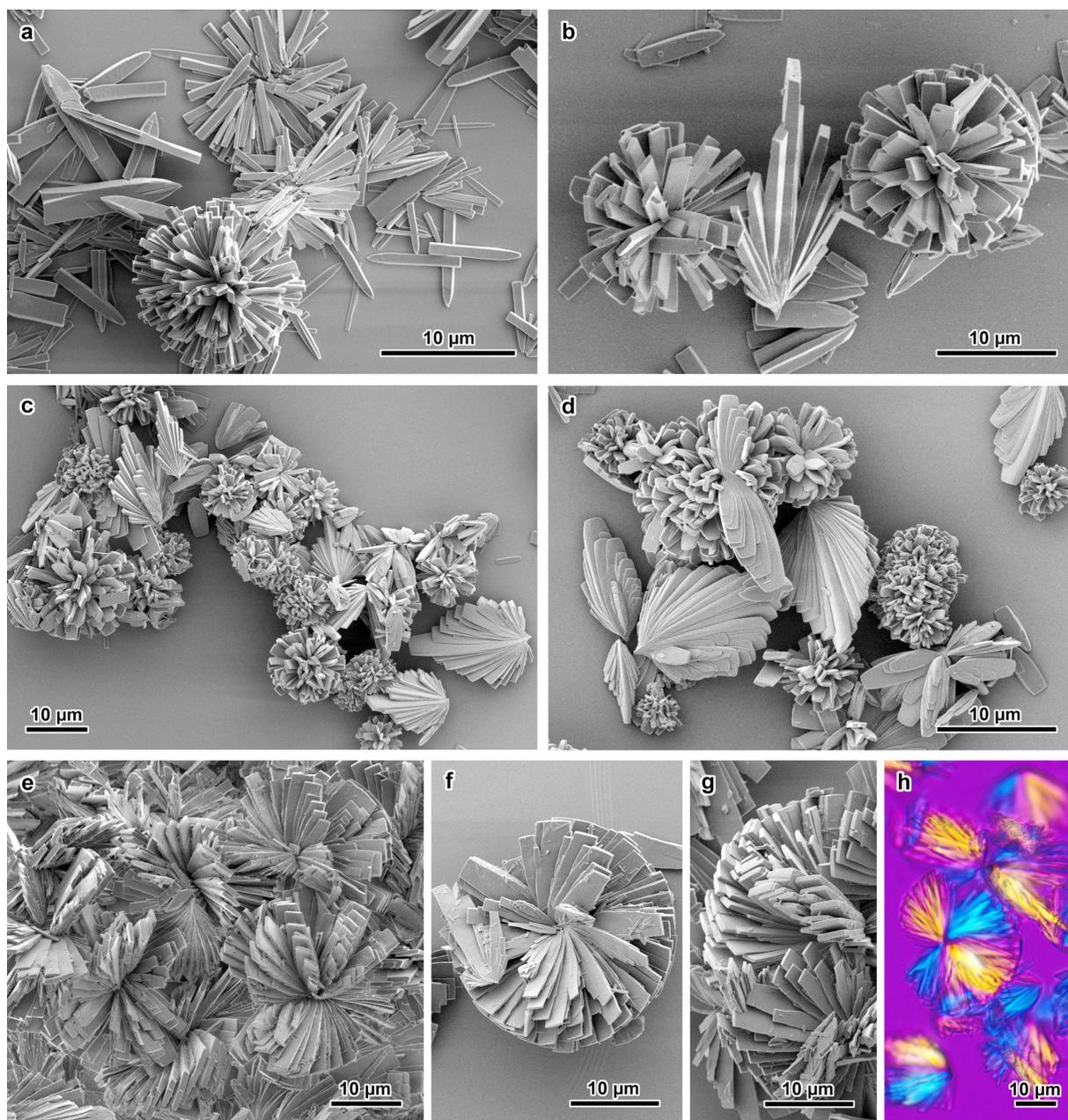
**Figure 5.** SEM images of the A-type amylose crystals prepared from fractions SAA14–21 at various concentrations at 0.3% w/v (a), 1.0% w/v (b), 2.0% w/v (c), 4.0% w/v (d), by diffusion of acetone vapor at 55 °C. e-h) Crystal assemblies formed by crystallizing fraction SAA14–21 at 5.0% w/v with liquid acetone at 55 °C. Image (h) is a polarized light optical micrograph recorded with a retarding  $\lambda$ -plate.
