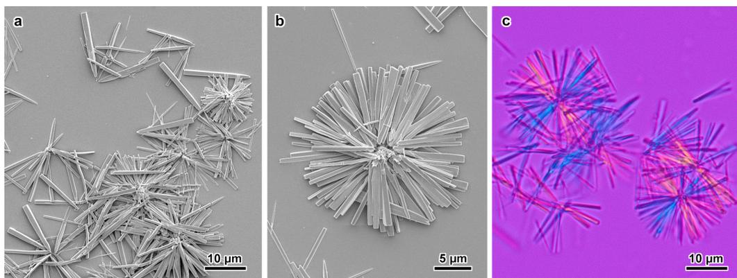
**Figure S1.** SEM images (a,b) and polarized light optical micrograph (c) of the single crystal assemblies observed by crystallizing fraction SAA14–21 at 0.05% w/v by diffusion of ethanol vapors at 60 °C. The image in (c) was recorded with a retarding  $\lambda$ -plate.
