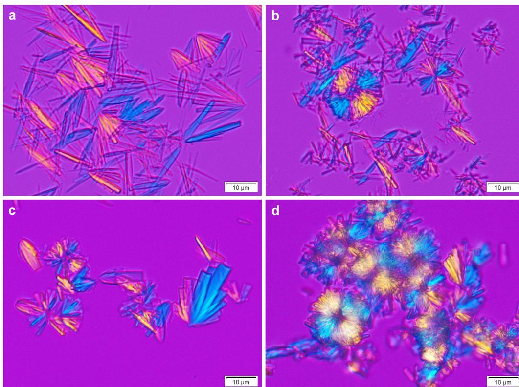
**Figure S2.** Influence of the initial concentration of SAA14–21 amylose fraction on the morphology of A-type crystals prepared by diffusion of acetone vapors at 55 °C: a) 0.05% w/v; b) 0.3% w/v; c) 1.0% w/v; d) 2.0% w/v. The polarized light optical micrographs were recorded with a retarding  $\lambda$ -plate.
