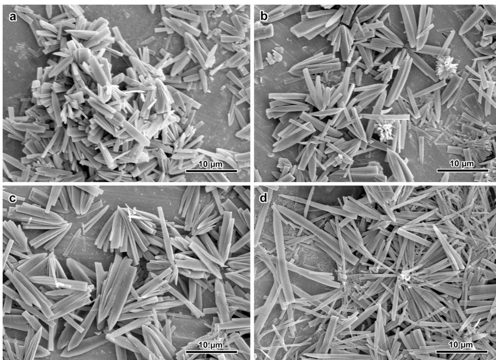
**Figure 2.** Influence of the crystallization temperature on the morphology of the A-type amylose single crystals prepared from fraction SAA14–21 (0.05% w/v) at 50 °C (a), 55 °C (b) and 58 °C (c) by diffusion of acetone vapors, and 60 °C (d) by diffusion of ethanol vapors (SEM images).
