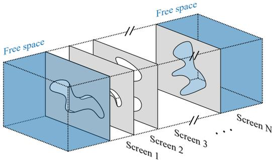
Figure 1: Unit cell of a multi-stacked FSS with perforated screens of arbitrary geometry.
