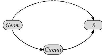
Figure 2: Different approaches to create a DL SM for characterizing a FSS. The dashed line depicts a model that directly relates the geometry ( $Geom$ ) of the FSS to its scattering parameters ( $S$ ), without making use of *a priori* knowledge. The solid line represents a SM that makes use of knowledge about the EM problem under study to establish an equivalent circuit as an intermediate step in the calculation of  $S$ .
