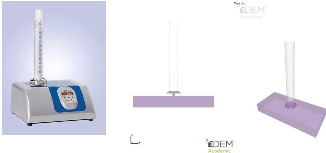
Figure 2. Pictures of the experimental Jolting Volumeter on the left (© Engelsmann) and the simulated by EDEM on the right (front and side views)
