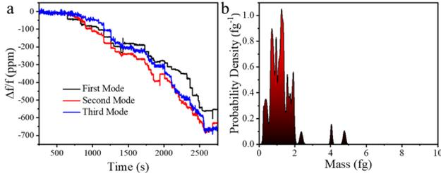
Figure 3: (a) Relative frequency shifts during the phage G experiments on a microcantilever resonator surface. (b) Mass probability density after applying the inverse problem algorithm.
