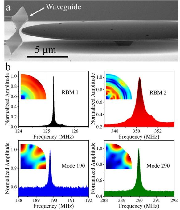
Figure 4: (a) Scanning electron microscope image of an optomechanical disk resonator of 11  $\mu\text{m}$  of radius used in this work. (b) Thermomechanical frequency response of the tracked modes measured in the nanomechanical mass spectrometer prototype. Inset: FEM simulation mode shape representation.
