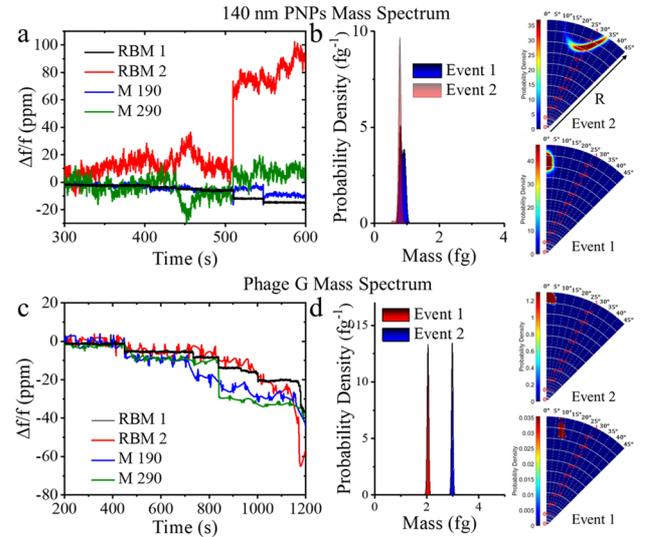
Figure 5: (a) Relative frequency shifts during the nebulization of 140 nm polystyrene nanoparticles. (b) Mass spectrum and landing position in polar plot representation obtained from two tentative events. (c) Relative frequency shift during the nebulization of phage G viral particles. (d) Mass spectrum and landing position in polar plot representation of two tentative events during the nebulization of phage G viral particles.
