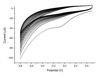
Figure 4 Cyclic voltammogram of PMeOx electrografting by electroreduction of the associated diazonium ( $5 \times 10^{-4}$  M in ACN with 20 eq of tBuNO<sub>2</sub> and 0.1 M of TBAPF<sub>6</sub> on ITO electrode Scan rate 0.1 V/s
