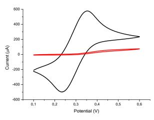
Figure 5 CVs of ferrocene  $(10^{-3} \text{ M} \text{ in acetonitrile with } 0.1 \text{ M} \text{ LiClO}_4)$  at 100 mVs<sup>-1</sup> before (black line) and after grafting of PMeOx on ITO electrode
