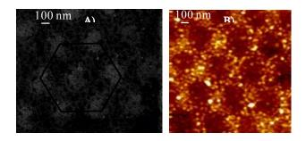
Figure 7 A) SEM image. B) AFM image of nano structured array of e Polyoxazoline layer on ITO obtained using 500 nm diameter PS sphere
