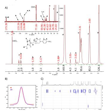
Figure 3: PnPrOX (Table 2, run 4): A) <sup>1</sup>H and <sup>13</sup>C NMR in CDCl<sub>3</sub> at 20°C; B) SEC trace: RI (red), UV (purple) at  $\lambda = 254$  nm; C) DOSY NMR in CDCl<sub>3</sub> at 298 K
