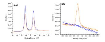
Figure 6 High-resolution XPS spectra of a gold surface, before (blue) and after (orange) polymer electrografting. a) high resolution  $Au_{4f}$  signals, b) high resolution  $N_{1s}$  signal
