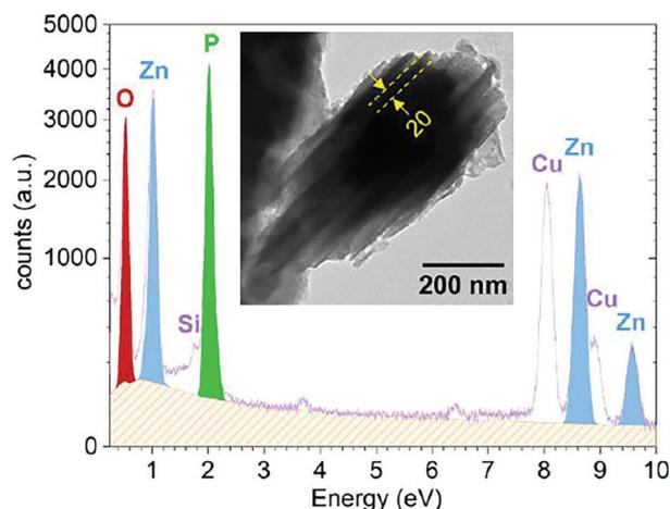
**Figure 3.** EDX spectrum of prismatic crystals made of Zn, P, and O. Cu signal is to originate from the TEM grid, growth substrate, and the film itself. The inset shows a TEM image of the flattened prismatic crystal of zinc phosphate hydrate, confirming its lamellar structure.
