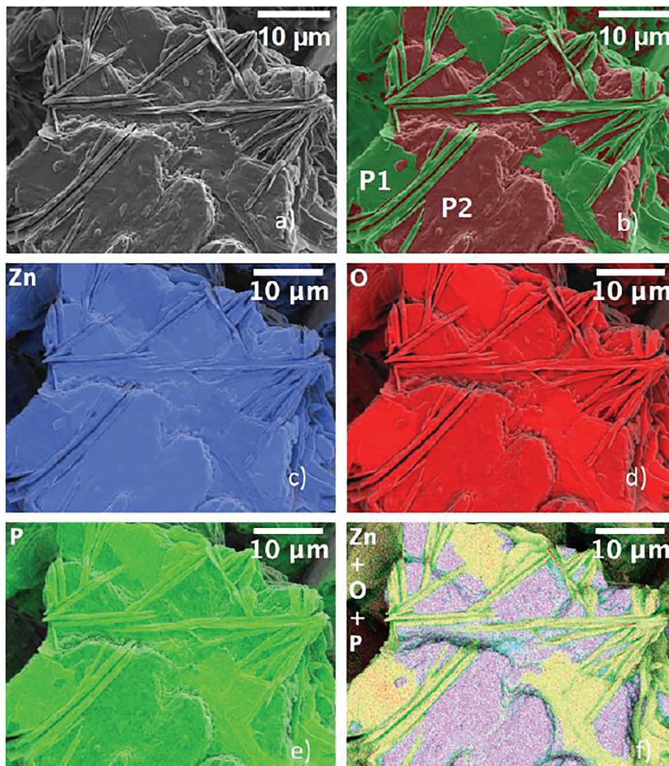
**Figure 2.** a) SEM image of the grown zinc phosphate film. (b–f) Elemental maps of zinc phosphate film: Zn (blue), O (red), P (green), Zn+O+P and chemical phase mapping of hydrated phase P1  $\{Zn_3(PO_4)_2 \cdot 4H_2O$  and/or  $Zn_3(PO_4)_2 \cdot 2H_2O\}$  and pyrophosphate phase P2 ( $Zn_2P_2O_7$ ).
