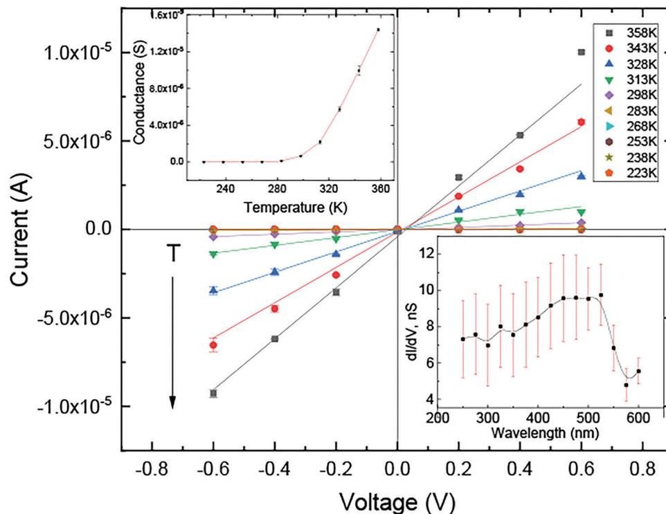
**Figure 5.** Current-voltage characteristics of the films obtained at varying  $T$  of  $\approx 223$ – $358$  K. The inset shows conductance versus  $T$  plot, and the data were fitted with Arrhenius expression yielding  $E_a$  of  $285 \pm 8$  meV. The plot of intensity-normalized differential conductance versus light wavelength obtained at  $\approx 0$  V is shown in the lower left inset.
