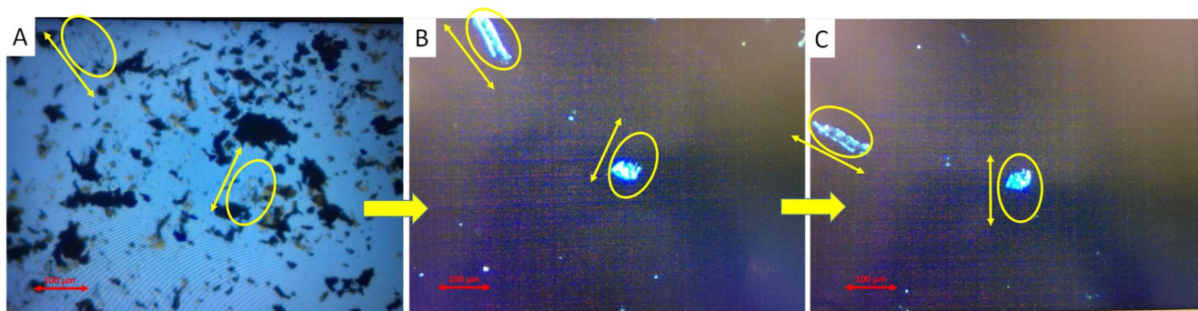
Figure 13: polarised light study of thin C 2 N flakes (yellow circles). A): normal light; B): same flakes under cross polarized light and C) same sample upon rotation. The appearance of the flakes alternatively goes brighter and darker as a function of the angle.
